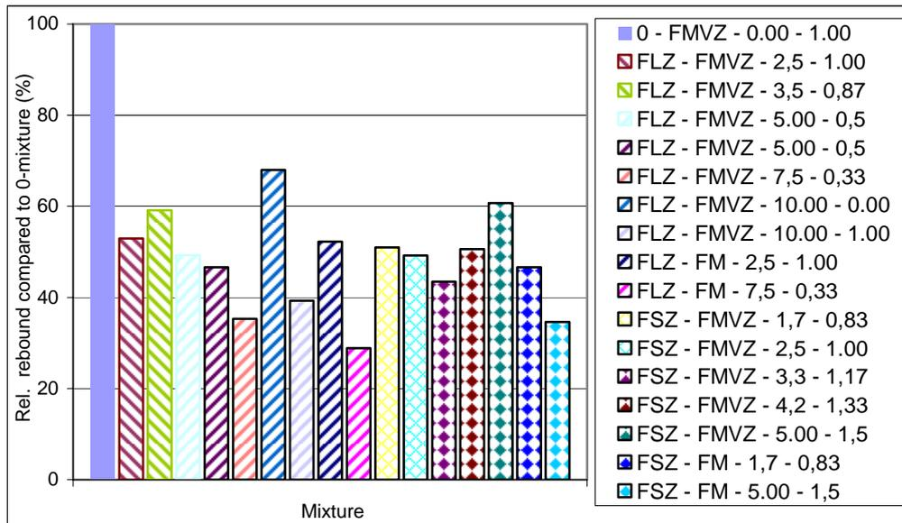
Figure 2: Relative rebound compared to 0-mixtures
