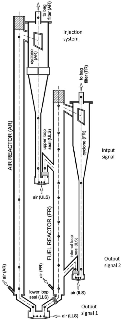
Figure 3: Cold flow model scheme indicating the main parts and the location of measuring coils and of the injection system. AR: 50mm internal diameter and 1.3m height, FR: 54mm internal diameter and 1m height.
