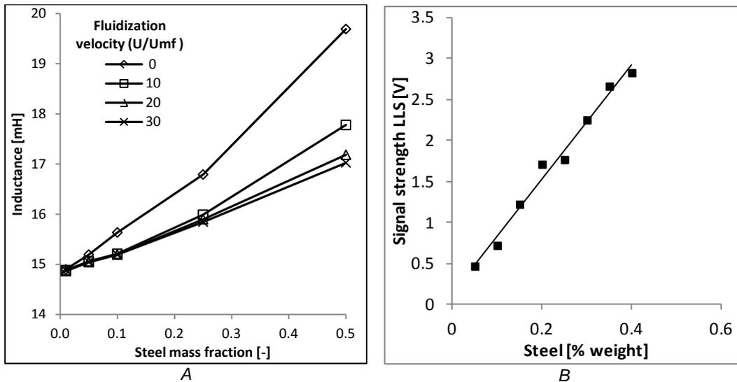
Figure 2: A: Inductance measured with LC resonator at fixed bed and fluidized bed conditions for different compositions of bronze/steel mixtures. B: Signal strength in volts measured by impedance method for different concentration of ferromagnetic particles.
