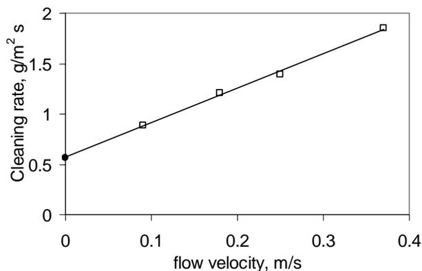
Fig. 11 Influence of velocity on the cleaning rate in pipes fouled with WPC gels. The empty square points and line are taken from the study by Xin *et al.* (2004) using 0.5 wt% NaOH at 65°C. The solid square is  $R_0$  estimated for a standard HIG dissolved at the same conditions, assuming no velocity effects.
