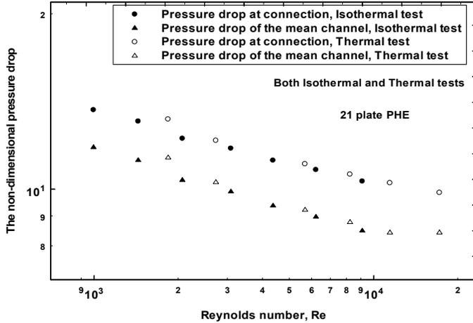
Fig. 7 Comparison of the experimental pressure drop of both isothermal and thermal tests for the connection and the mean channel for a 21 plate package plate heat exchanger.
