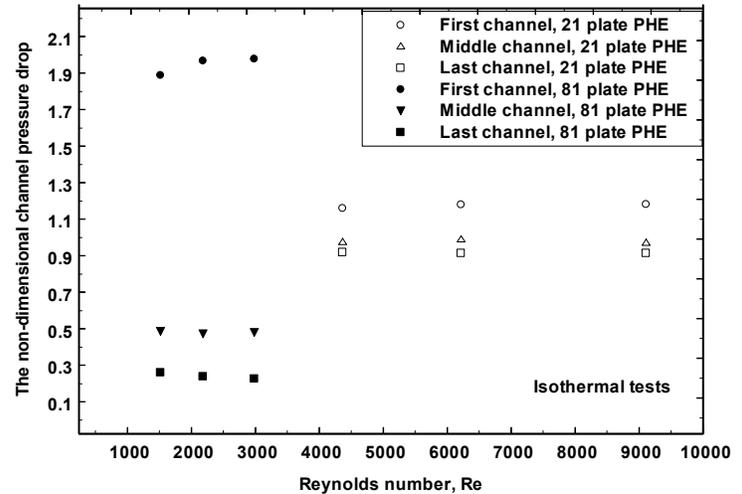
Fig. 9 Comparison of the channel pressure drop between a small and a large plate package plate heat exchanger.
