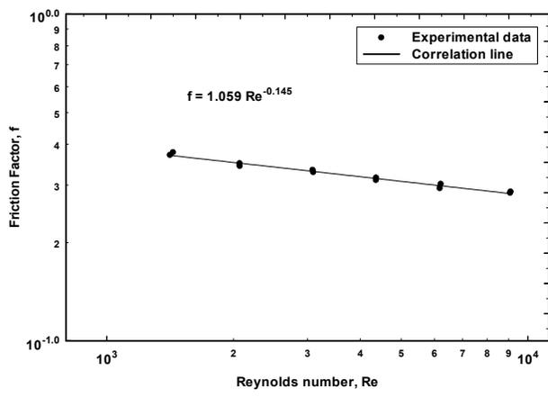
Fig. 5 Flow friction characteristics of chevron plate (the corrugation angle,  $\beta=30^\circ$ )
