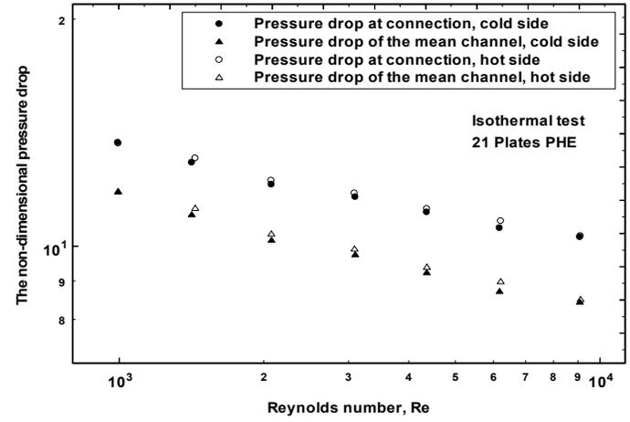
Fig. 6 Comparison of the experimental pressure drop between the connection and the mean channel for a 21 plate package plate heat exchanger.
