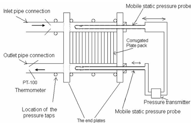
Fig. 4 Various locations of the fixed the pressure taps, the differential pressure transmitter and PT-100 thermometer across the tested plate heat exchanger.
