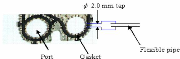
Fig. 3 Arrangement of the pressure tap of the channel in the tested plate heat exchanger.
