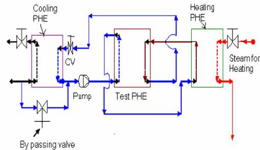
Fig. 2 The detailed circuit of cold and hot fluids
