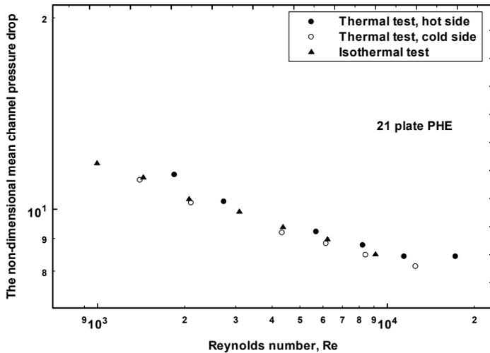
Fig. 8 Comparison of the mean channel pressure drop of isothermal and non-isothermal tests.
