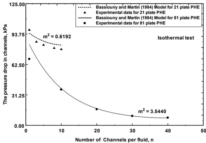
Fig. 10 Comparison of the experimental channel pressure drop with Bassiouny and Martin (1984a) analytical model in a small and a large package plate heat exchanger.
