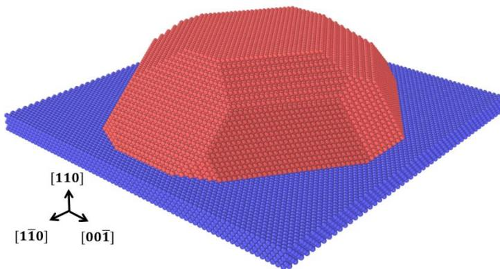
Figure 1 – A faceted Fe nanoparticle on a hard substrate in MD simulations (taken from [2]).
