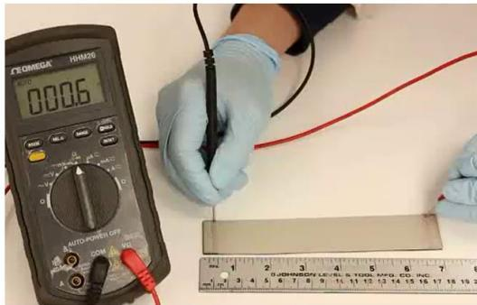
Figure 1 - Resistivity measurement ( $\sim 0.6\Omega$ ) of hybrid conductive coating on top of composite laminate
