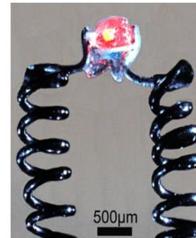
Figure 3 - Conductive structure (PLA with 5w MWCNTs)
