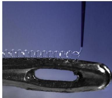
Figure 2 - Microstructured fibers printed on top of a sewing needle
