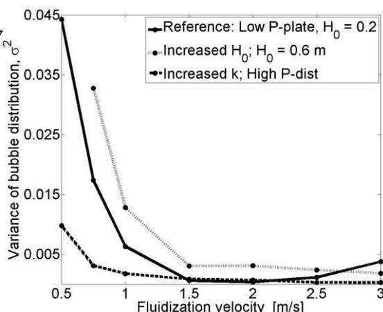
**Figure 7:** Variance of bubble distribution as a function of fluidization velocity. Reference conditions: Low  $\Delta p$ -plate and  $H_0 = 0.2$  m.
