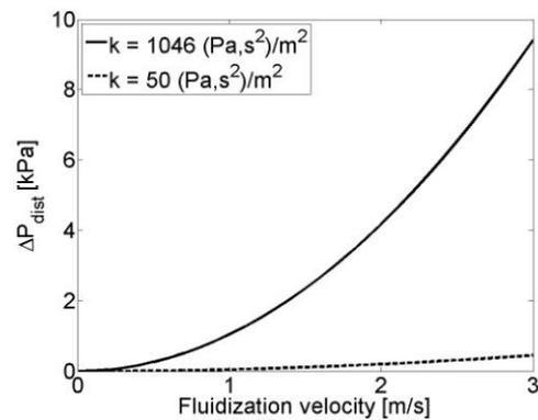
Figure 3:  $\Delta p-u$  curves for the gas distributors used in the experiments
