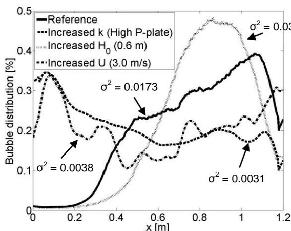
**Figure 6:** Bubble distribution profile as obtained from DIA. Reference conditions: Low  $\Delta p$ -plate,  $H_0 = 0.2$  m and  $u = 0.75$  m/s.
