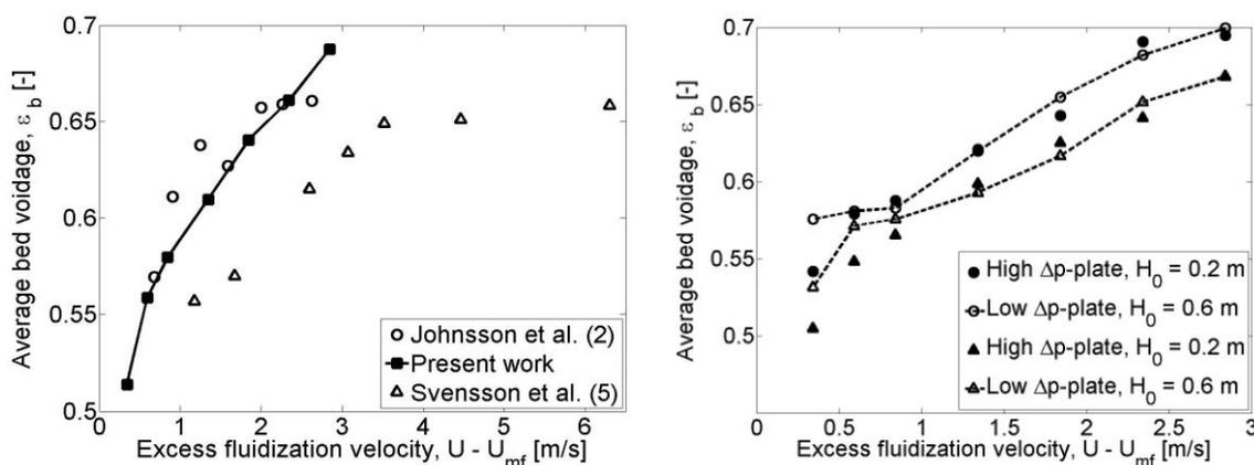
a) Values from present work (solid line with markers) and from literature. b) Bed voidage from this work for two different bed heights and distributor plates.
