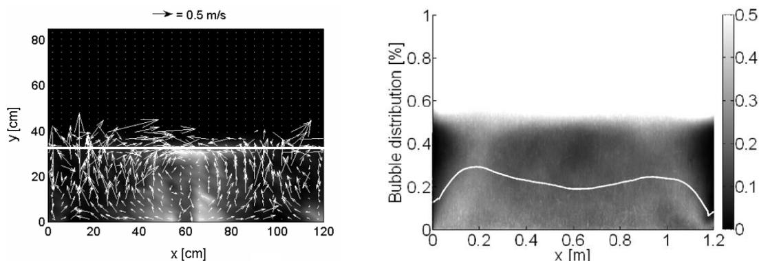
a) Fuel mixing flow pattern. Tracer concentration (gray field) and tracer velocity (vector plot). From Pallarès *et al.* (2) with permission,  $H_0 = 0.33$  m,  $u = 0.7$  m/s,  $k = 1046$  Pa\*s<sup>2</sup>/m<sup>2</sup>.
