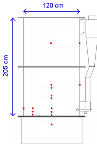
Figure 2: The cold 2-D FB unit used in the experiment. Pressure taps marked with dots
