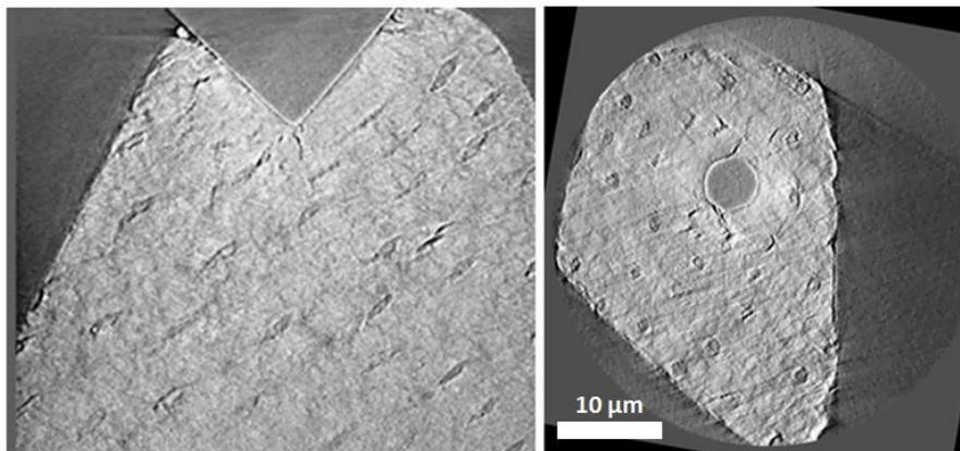
Figure 1 – Virtual cross sections of the nanoindentation of elephant dentin, acquired using a nanoscale X-ray microscope. Crack development around the indenter tip, as well as the neighboring tubule structures, can be observed and contributes to the material's fracture toughness.
