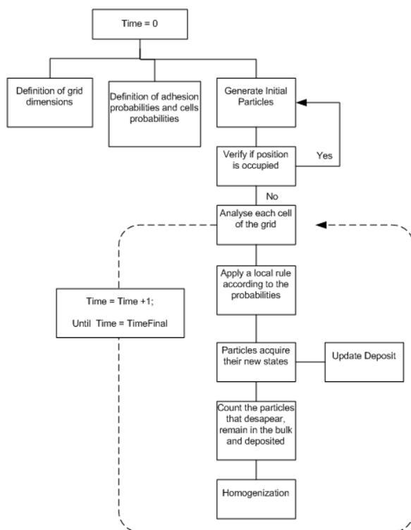
Figure 5 – Workflow of the software tool.
