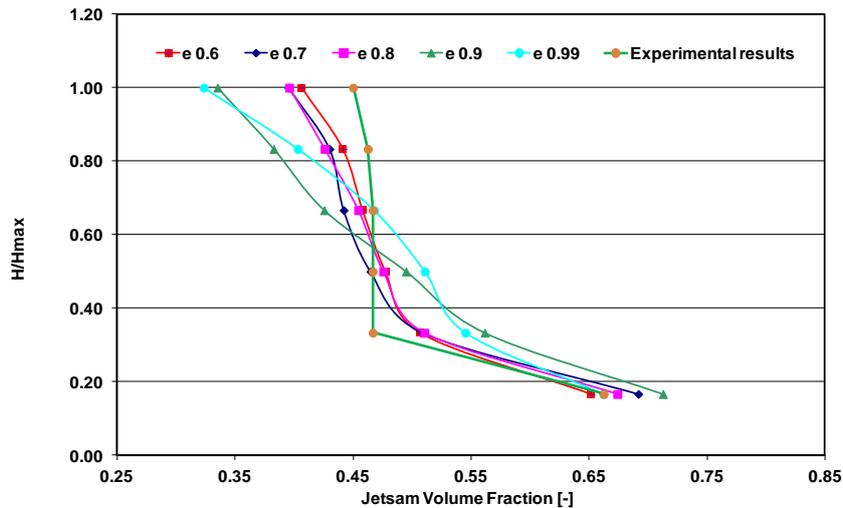
**Figure 3.** Stationary axial profiles of average jetsam volume fraction as a function of restitution coefficient. The superficial fluid velocity is 0.10 m/s. FUS. Comparison with the experimental results.
