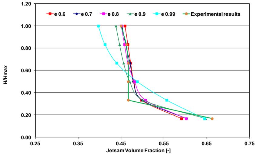
**Figure 6.** Stationary axial profiles of average jetsam volume fraction as a function of restitution coefficient. The superficial fluid velocity is 0.10 m/s. SUS. Comparison with the experimental results.
