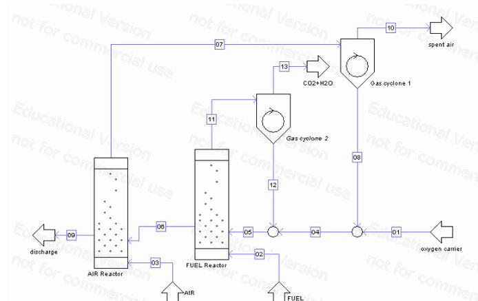
Figure 4: Flowsheet of CLC process in SolidSim
