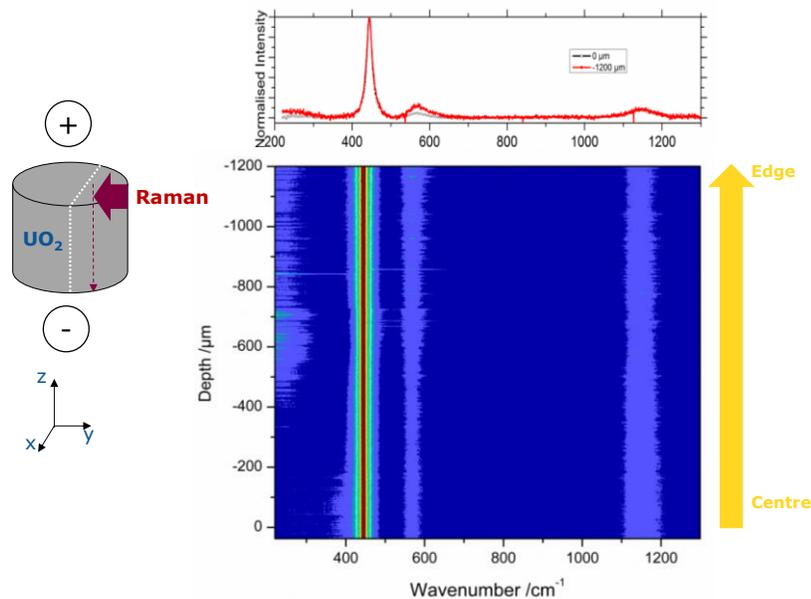
Figure 1 – Raman mapping of  $\text{UO}_2$  pellet made by SPS indicating a gradient in the oxidation state.
