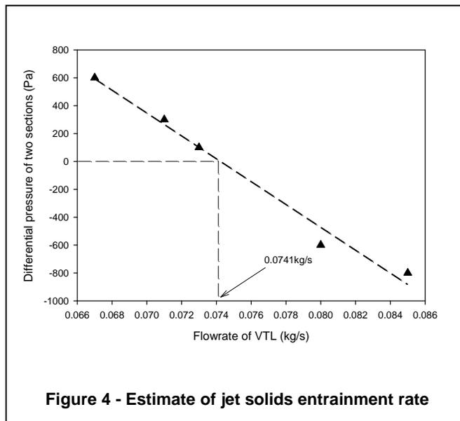
In practice, it was difficult to exactly achieve a steady differential pressure of 0 between the two compartments. Several experiments were, therefore, conducted with different gas flows to the VTL
