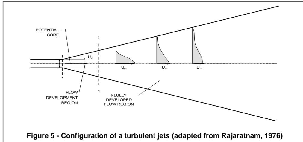
As for turbulent jets in conventional fluids, jets in fluidized beds have a “potential” core within which gas momentum, temperature and composition are the same as at the mouth of the orifice. Merry suggested a scheme of the particle tracks in the vicinity of the jet, shown in Figure 6, with the majority of entrainment occurring near the nozzle tip in the potential zone region [Merry, 1971].
