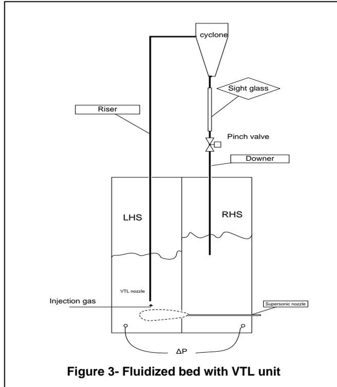
of bed to the right side through the VTL, while solids were conveyed back from the right side to left side by the supersonic nozzle through the draft tube connecting the two compartments. Coke particles, with a Sauter mean diameter of 135  $\mu\text{m}$  and a density of 1450  $\text{kg/m}^3$ , were used for the study. Several convergent-divergent supersonic nozzles, of various dimensions, were tested.
