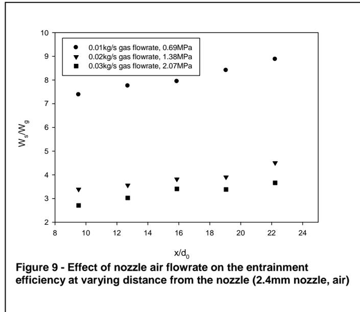
Figure 9 - Effect of nozzle air flowrate on the entrainment efficiency at varying distance from the nozzle (2.4mm nozzle, air)
