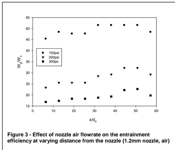
Figure 3 - Effect of nozzle air flowrate on the entrainment efficiency at varying distance from the nozzle (1.2mm nozzle, air)
