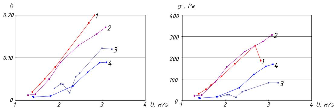
Fig. 5. The dependence graphs of  $\delta$  (a) and  $\sigma$  (b) excess according to the air velocity (1 – culm100%, 2 – culm 80%, straw pellets 20%, 3 – culm 50%, straw pellets 20%, 4 – culm 20%, straw pellets 80%).
