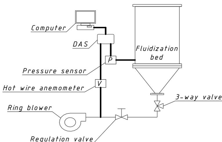
Fig. 1. – Scheme of an experimental device
