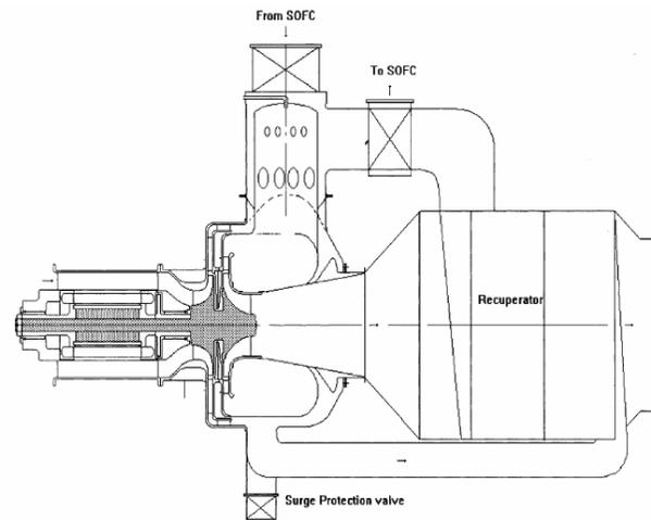
Fig. 2 Microturbine system with a rear-mounted recuperator (McDonald, 2003).
