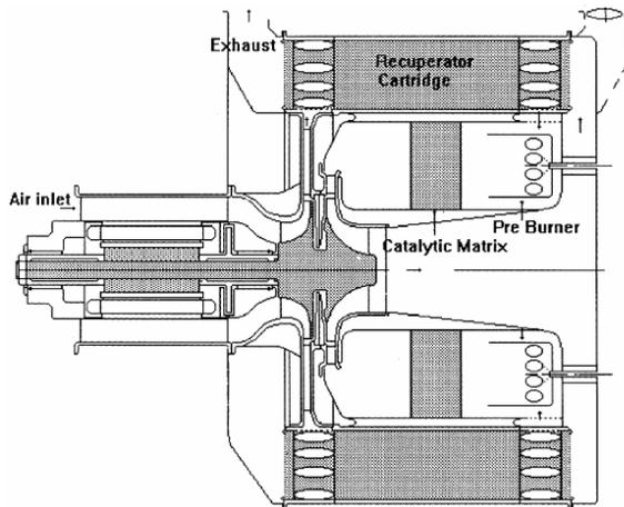
Fig. 1 Microturbine system with an annular wrap-around recuperator (McDonald, 2003).
