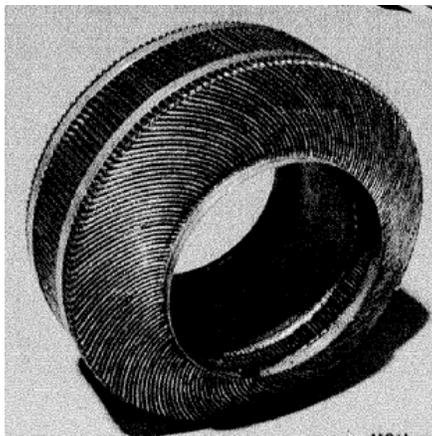
Fig. 5 Annular primary surface stainless steel recuperator from Solar Turbines, Inc. (Treece et al., 2002).
