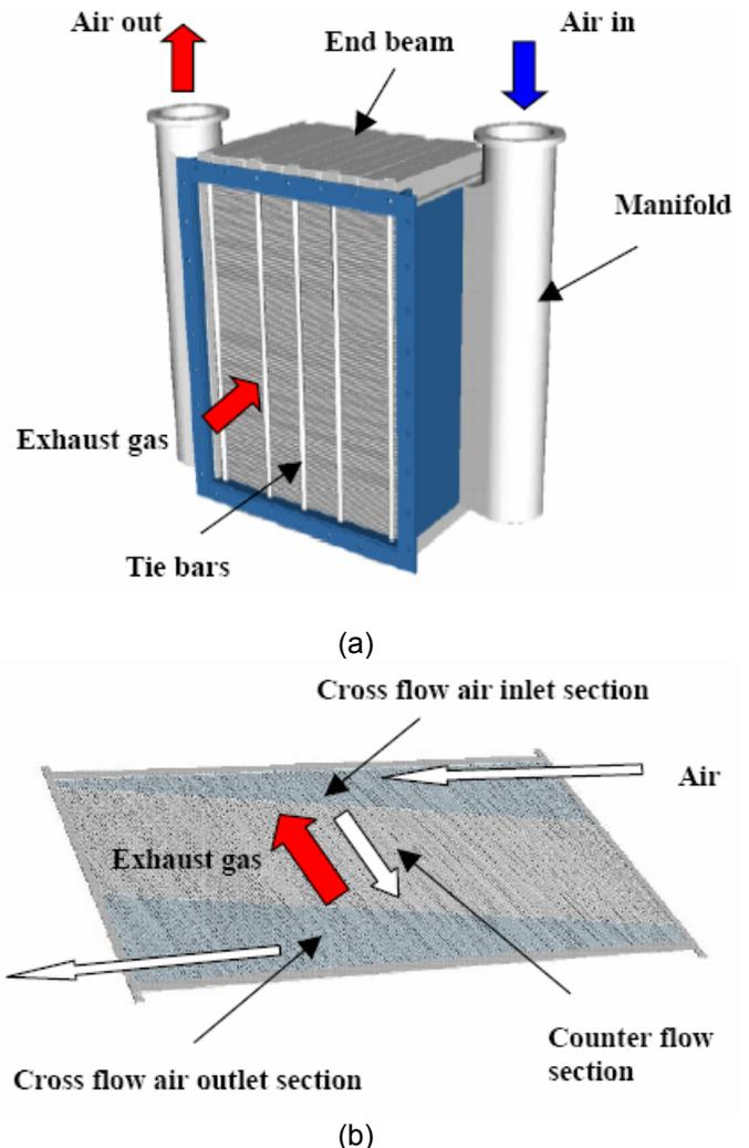
Fig. 6 (a) Primary surface recuperator, and (b) a typical air passage geometry (Lagerström and Xie, 2002).
