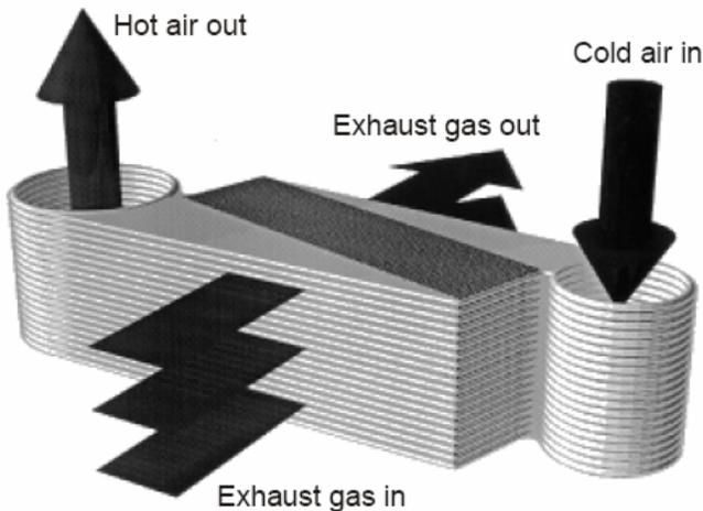
Fig. 10 Recuperator sketch showing flow paths. Manifolds for cold air entering and hot air leaving the recuperator are created by welded circular flanges (Kesseli et al., 2003).
