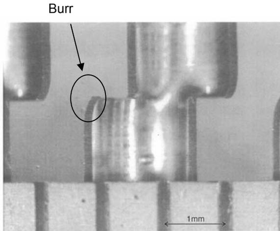
Figure 6 Cross Section of the Fin
