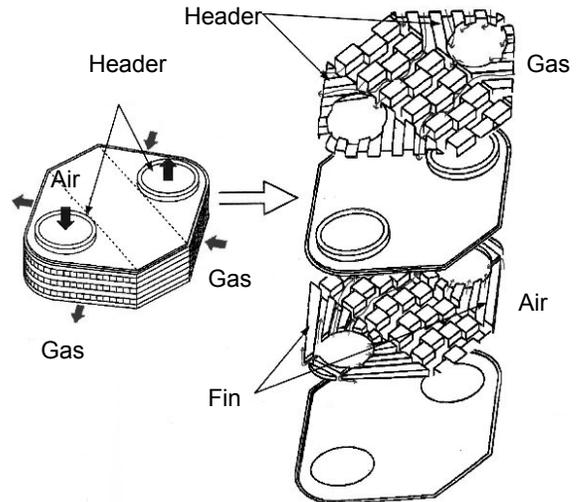
**Figure 1 Structure of the Heat Exchanger**
