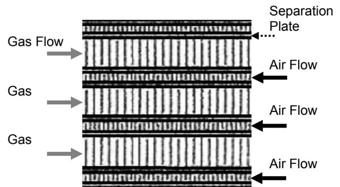
**Figure 2 Cross Section of Main Heat Exchanging Zone**
