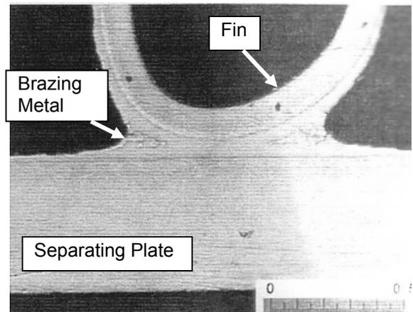
Figure 7 Joined Zone of the Fin
