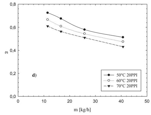
Figure 4: Effectiveness as a function of air mass flow at different temperatures: a) clean; b) 10 PPI; c) 20 PPI; d) 30 PPI
