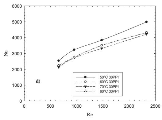
Figure 3: Nusselt number as a function of Reynolds number at different temperatures: a) clean; b) 10 PPI; c) 20 PPI; d) 30 PPI
