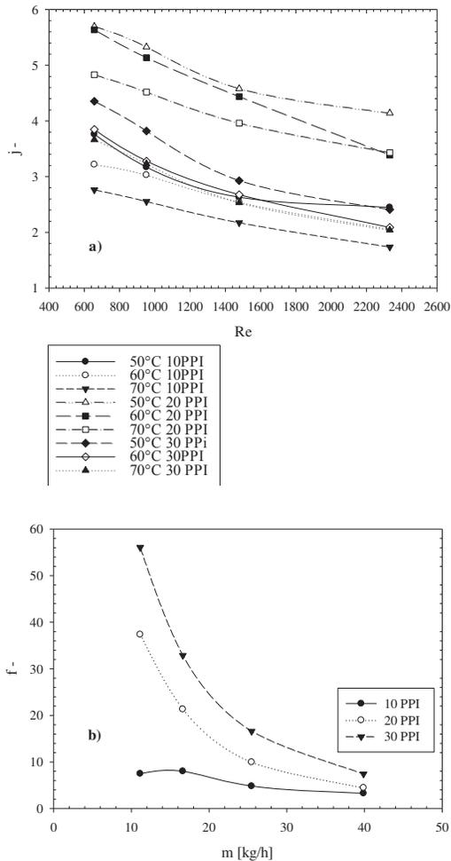
Figure 5: a) Colburn factor as a function of Reynolds number; b) friction factor as a function of air mass flow rate.
