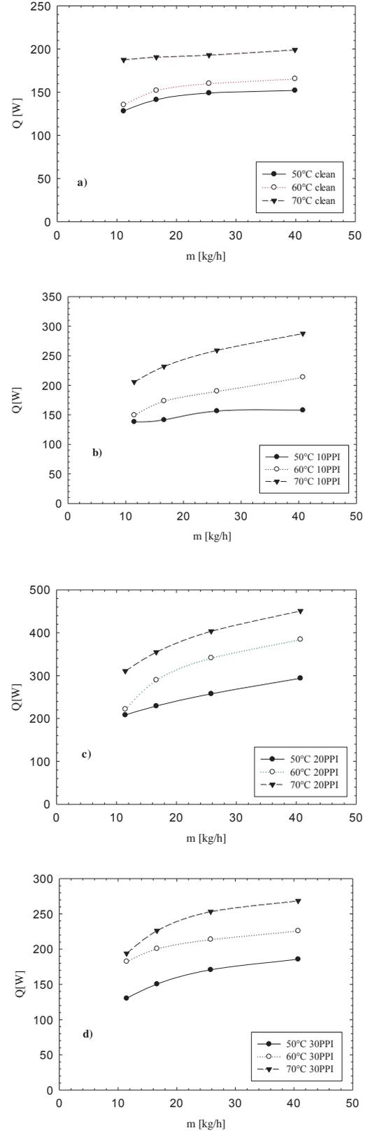
Figure 2: Heat transfer rate as a function of air mass flow at different temperatures: a) clean; b) 10 PPI; c) 20 PPI; d) 30 PPI
