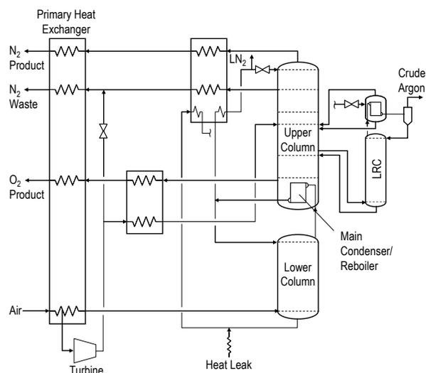
Figure 1. Air Separation Plant Flowsheet
