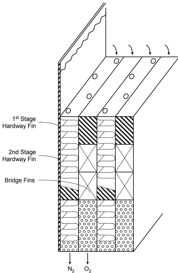
**Figure 14. Flow Distribution Technique Employed by Srinivasan et al (1995)**
