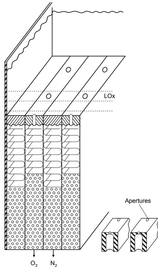
**Figure 10. Flow Distribution Technique Employed by Petit et al. (1986) (Design 1)**
