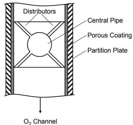
**Figure 13. Flow Distribution Device Employed by Beduz et al. (1991)**
