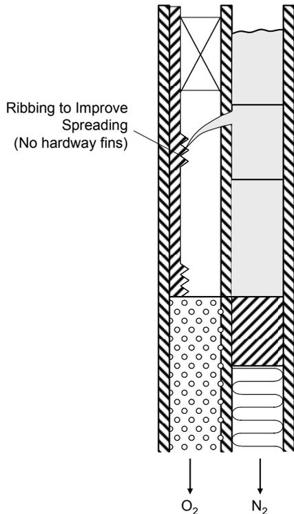
**Figure 11. Flow Distribution Technique Employed by Petit et al. (1986) (Design-2)**
