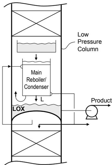
Figure 5. Once-Through Downflow Reboiler
