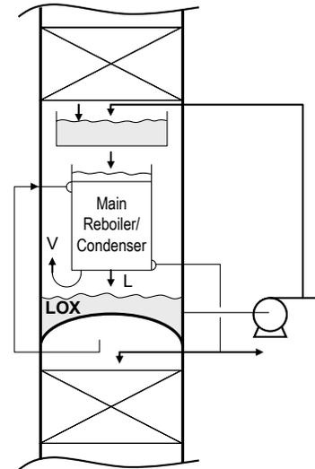
Figure 7. Recirculating Downflow Reboiler (Option 2)
