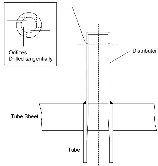
**Figure 15. Flow Distribution for Highflux Shell-and-Tube Main Condenser/Reboiler**
