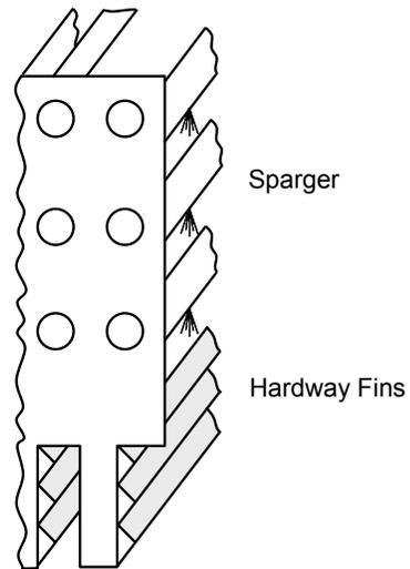
**Figure 12. Flow Distribution Device Employed by Swaminathan et al. (1992)**
