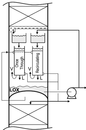
Figure 6. Recirculating Downflow Reboiler (Option 1)
