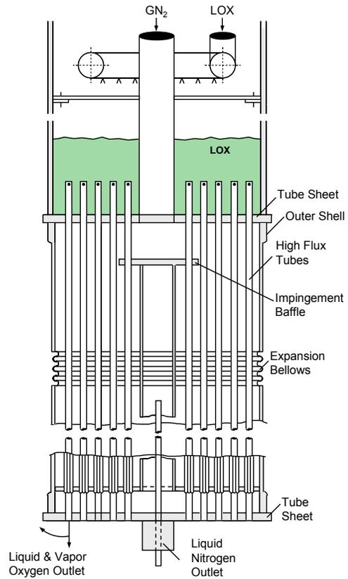
Figure 3. Shell-and-Tube Downflow
