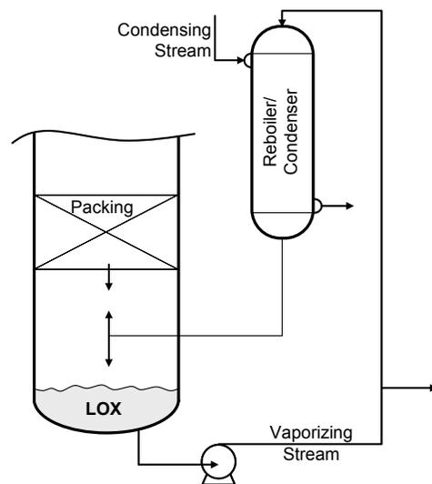
Figure 8. Recirculating Downflow Reboiler (Option 3)
