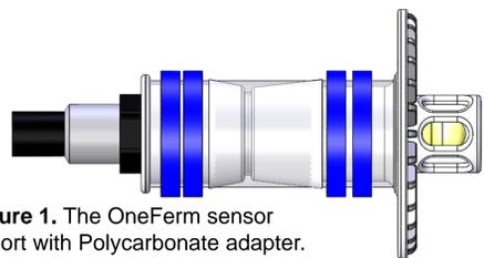
Figure 1. The OneFerm sensor in port with Polycarbonate adapter.
