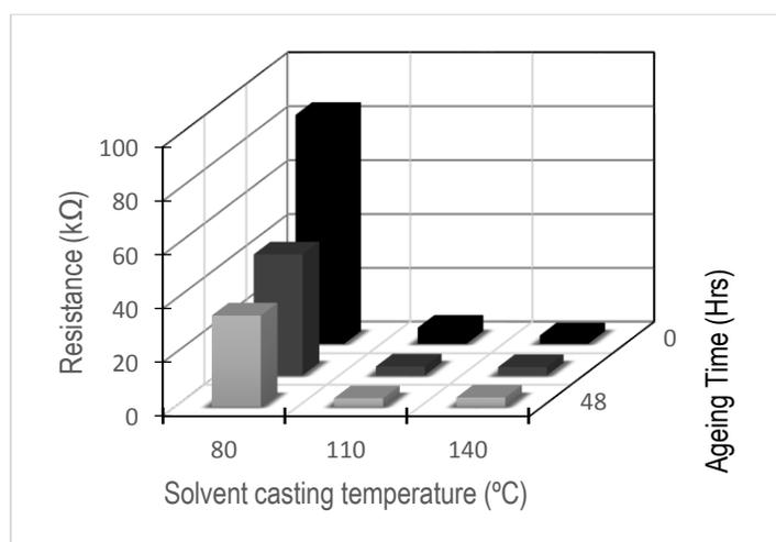
Figure 1 – effect of solvent casting temperature and ageing time on the electrical resistance of PHB/Graphene nanocomposite
