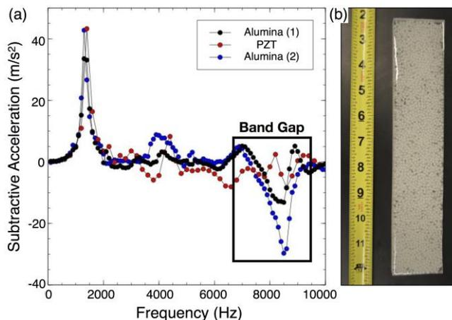
Figure 1 – (a) Subtractive acceleration as a function of frequency for acoustic metamaterials samples with different core-resonator materials. (b) Photograph of an acoustic material sample composed of acoustic resonators randomly dispersed in an epoxy matrix.
