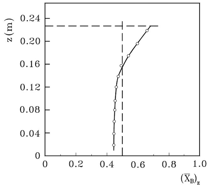
Figure 7. Average value of weight fraction of the particles of greater density, at different levels. System: binary mixture of 50 wt % of glass beads and of 50 wt % wood beads of particle diameter  $d_p = 3$  mm,  $\gamma = 45^\circ$ ;  $D_o = 0.04$  m;  $H_o = 0.24$  m.
