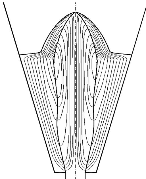
Figure 5. Solid trajectories in the whole bed. Experimental conditions:  $\gamma = 45^\circ$ ,  $D_o = 0.03$  m,  $H_o = 0.18$  m, glass beads of  $d_p = 3$  mm,  $u = 1.02 u_{ms}$ .
