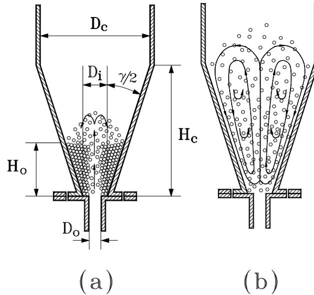
Figure 2. Geometric factors of the conical contactor and particle states in the spouted bed regime (a) and in the dilute spouted bed (jet spouted bed) regime (b).
