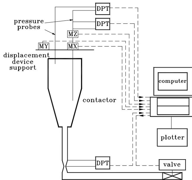
Figure 3. Schematic representation of the equipment and of the sampling device
