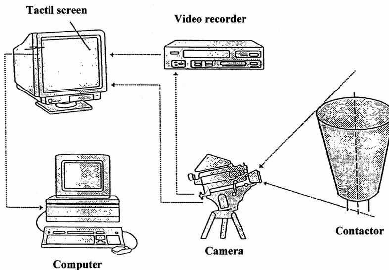
Figure 4. Scheme of the image treatment system.
