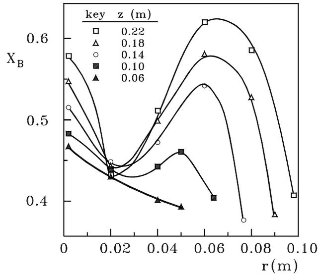
Figure 6. Weight fraction of the particles of greater density,  $X_B$ , at different radial and longitudinal position of the bed. System binary mixture (50 wt % of glass beads and wood beads of particle diameter  $d_p = 3$  mm).
