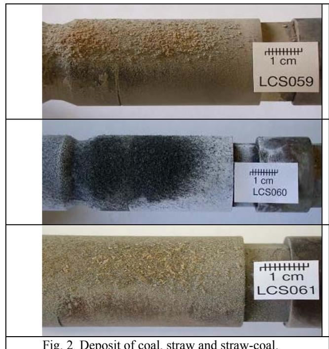
Fig. 2 Deposit of coal, straw and straw-coal.
