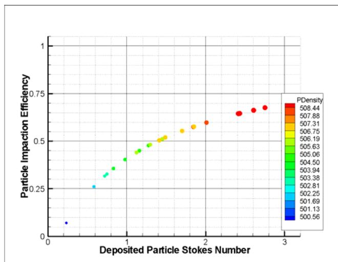
Fig. 9 ADP simulation with 500 kg/m<sup>3</sup> ash particles. Particle impaction efficiency vs particle Stokes number.
