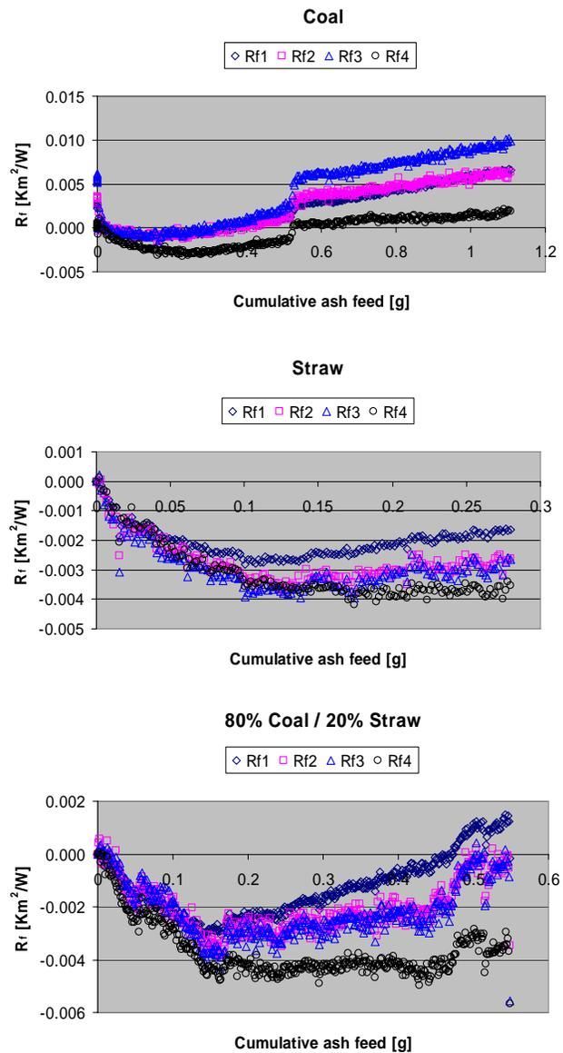
Fig. 5 Fouling factor  $R_f$  calculated from measured heat fluxes.  $R_f$  has been plotted against the mass of ash fed to the combustor with the fuel.
