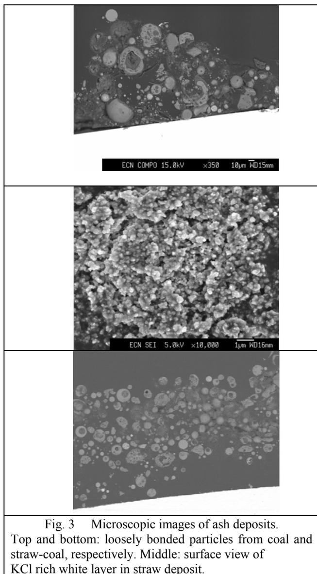
Fig. 3 Microscopic images of ash deposits. Top and bottom: loosely bonded particles from coal and straw-coal, respectively. Middle: surface view of KCl rich white layer in straw deposit.
