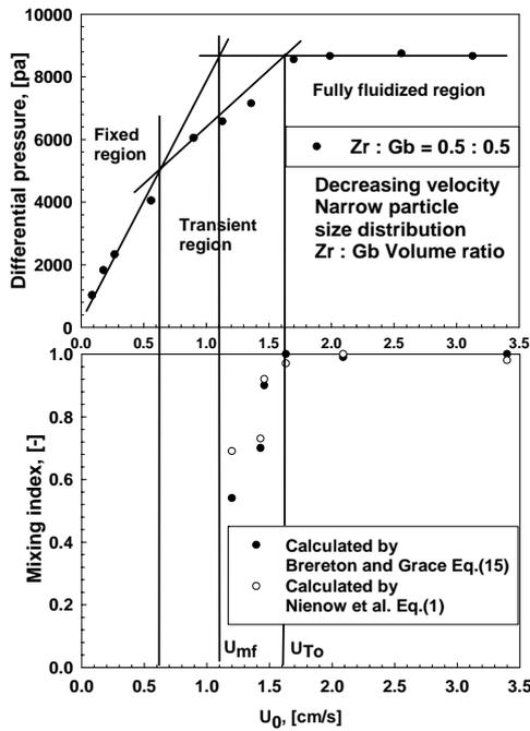
Fig. 6 Fluidization region according to superficial gas velocity.
