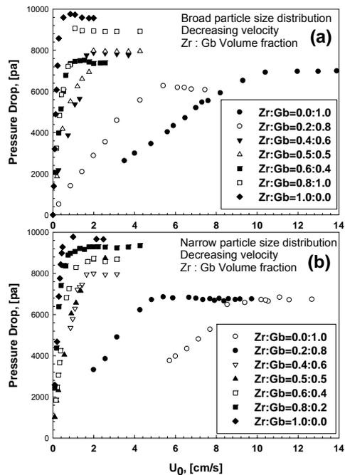
Fig. 2 Differential pressure vs. superficial gas velocity of (a) Binary solids with broad particle size distribution and (b) Binary solids with narrow particle size distribution.
