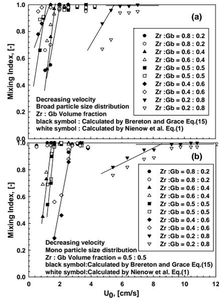
Fig. 7 Solid mixing index according to decreasing superficial gas velocity of (a) Broad particle size distribution and (b) Narrow particle size distribution
