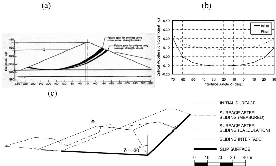
**Figure 3.** First slide. (a) The slip surface as predicted by Seed et al (1975), (b) critical acceleration coefficient for relative motion at the initial and final configurations in terms of the interface angle and (c) initial slide configuration assumed, computed final configuration and measured final configuration.
