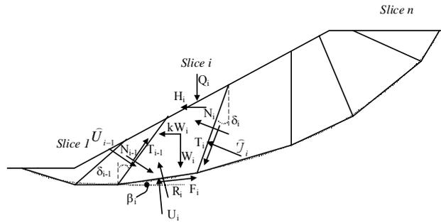
**Figure 1.** The multi-block stability method proposed by Sarma (1979).
