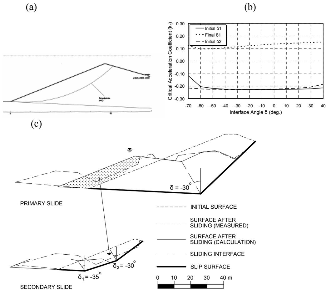
**Figure 5.** Second slide. (a) The slip surface as predicted by the Bishop stability method, (b) the critical acceleration coefficient at the initial and final configurations in terms of the interface angles and (c) the initial slide configuration assumed, computed final configuration and measured final configuration. In (b) for each case the other interface angle equals its critical value.
