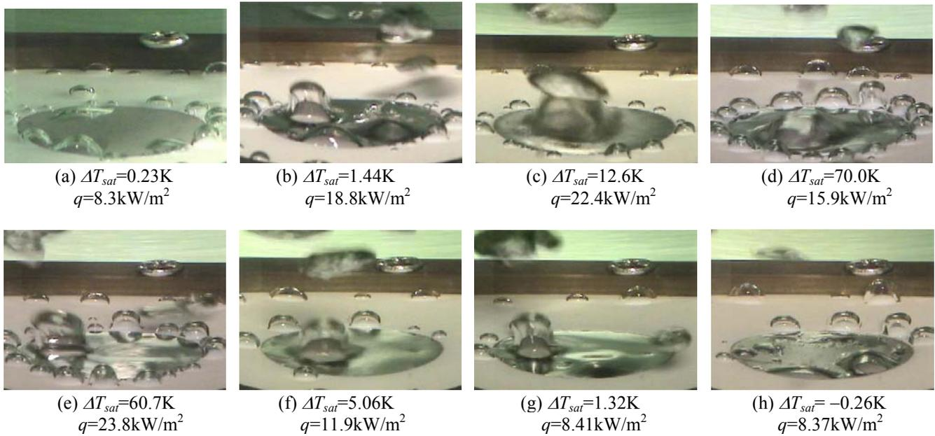
Figure 4: Behavior of bubble and vapor film in saturated boiling
