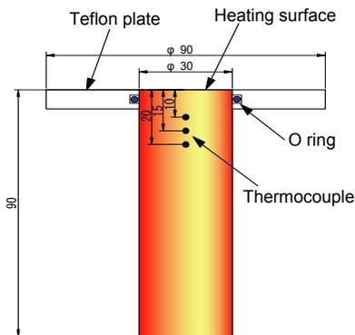
Figure 2: Heat transfer copper block
