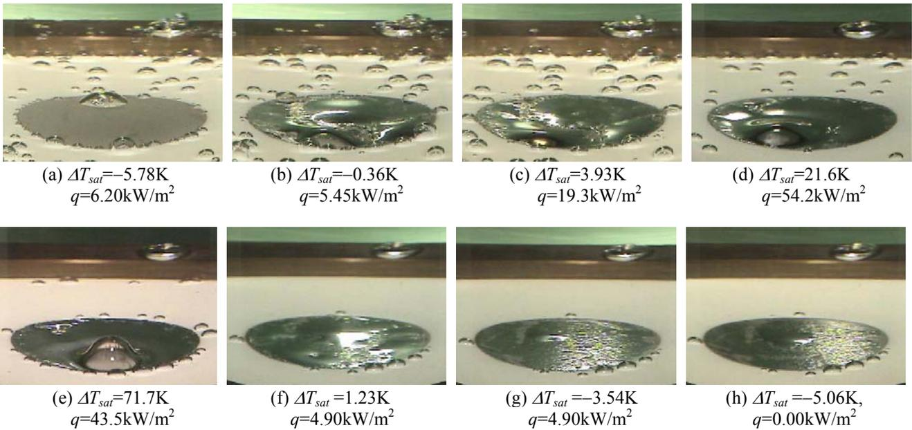
Figure 6: Behavior of vapor film for subcooling of 5K
