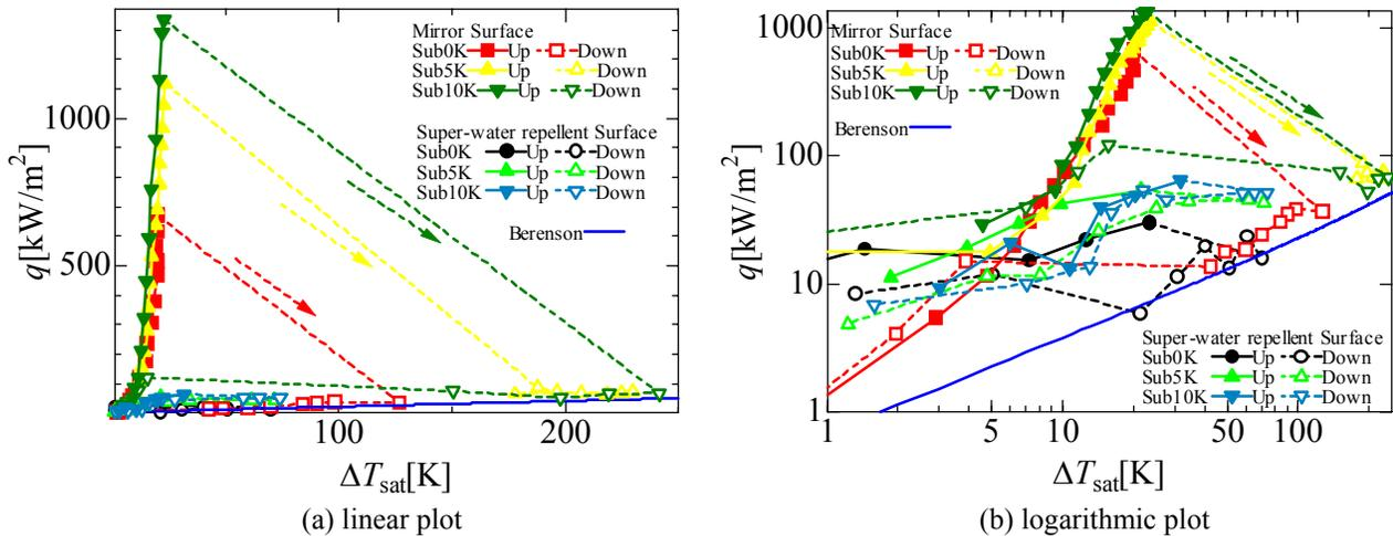
Figure 8: Heat transfer characteristic in subcooled boiling
