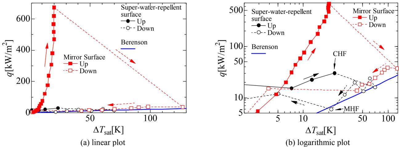
Figure 5: Heat transfer characteristic in saturated boiling
