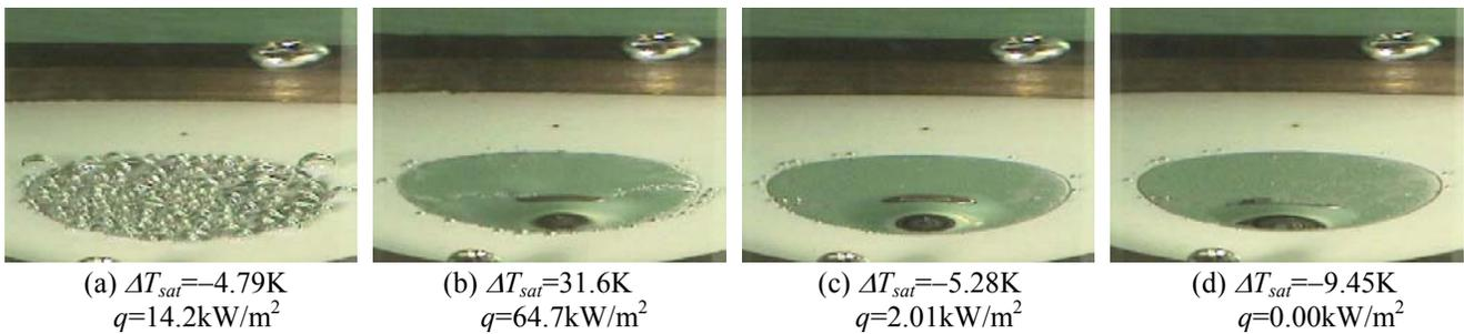
Figure 7: Behavior of vapor film for subcooling of 10K
