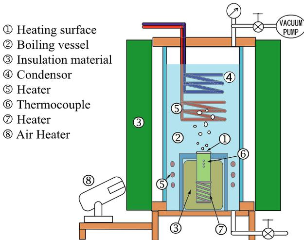
Figure 1: Experimental apparatus
