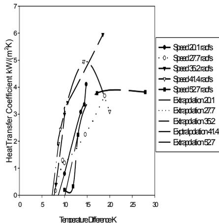
Figure 7. The effect of the rotational speed of the cone on the heat transfer coefficient for a Centritherm evaporator. Flow rate 0.025 kg sec. Temperature difference 10 °C.
