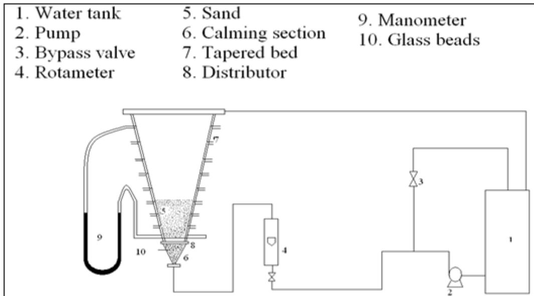
Figure 1. Schematic diagram of experimental set up.
