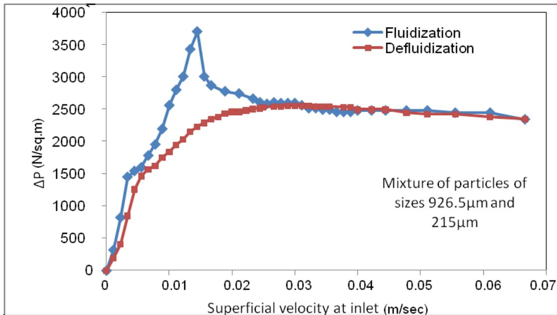
Figure 4 Characteristic plot of  $\Delta P$  against superficial velocity
