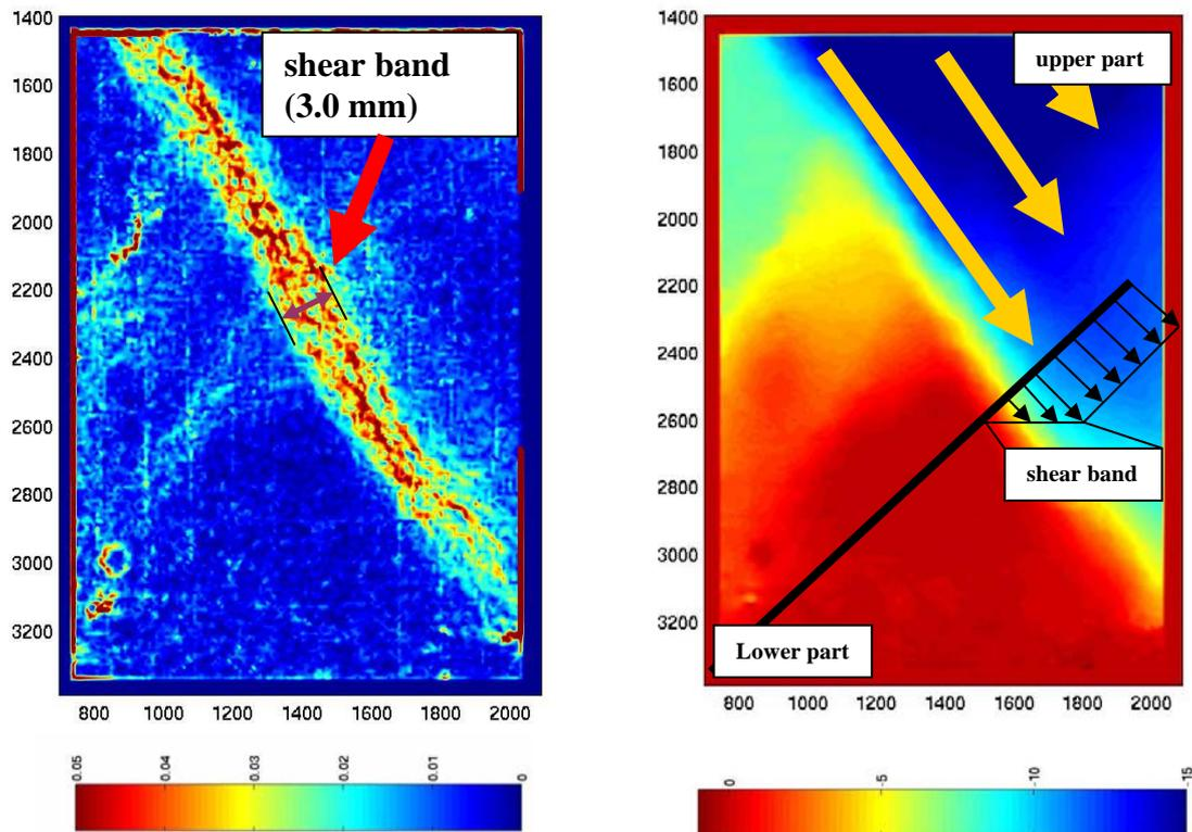
**Figure 2. Incremental shear strain (left) and total displacement (right) plot at 581-583 (Courtesy; Dr. Steve Hall, 2006, L3S, Grenoble)**
