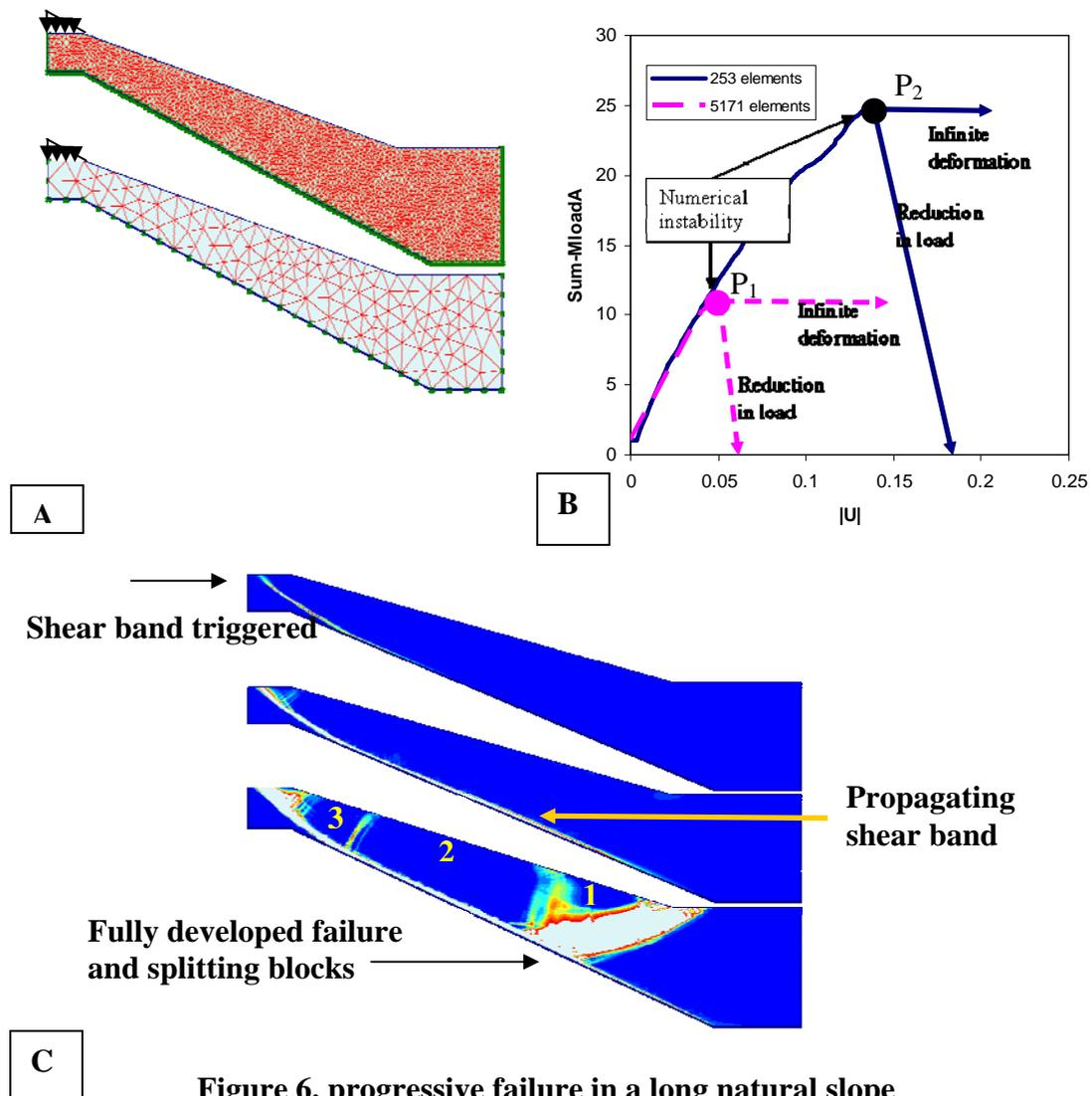
**Figure 6. progressive failure in a long natural slope**
