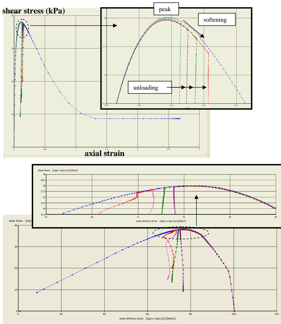
**Figure 4. Local shear stress-effective mean stress-axial strain response for the individual material point**
