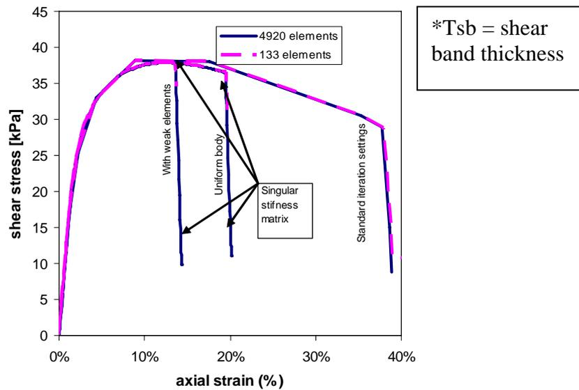
**Figure 5. Global response: shear stress versus axial strain**
