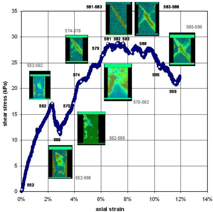
**Figure1. Plane strain biaxial stress strain relationship for the Norwegian Quick clay**
