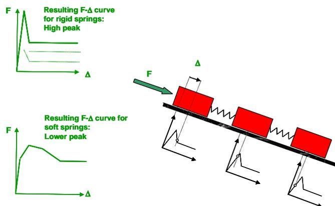
Figure 7. progressive failure mechanism (Nordal, 2004)
