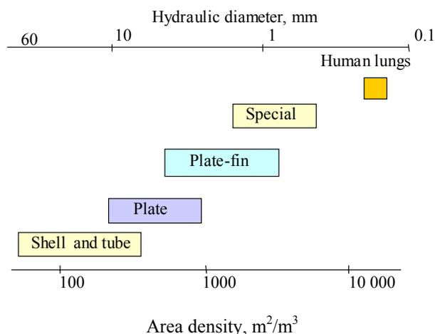
Fig. 1 Broad classification of industrial heat exchangers based on heat transfer area density and channel size
