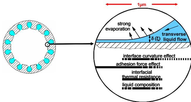
Fig. 7 Heat pipe evaporator and enlarged view of evaporation from thin liquid film with different microscale effects, adapted from (Stephan, 2002)
