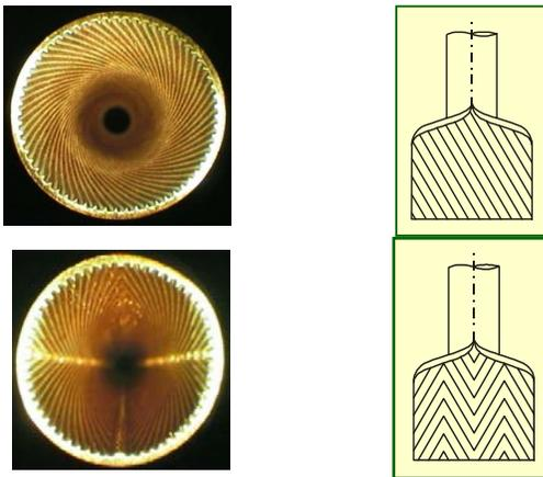
Fig. 5 Two types of microfin tubes.
