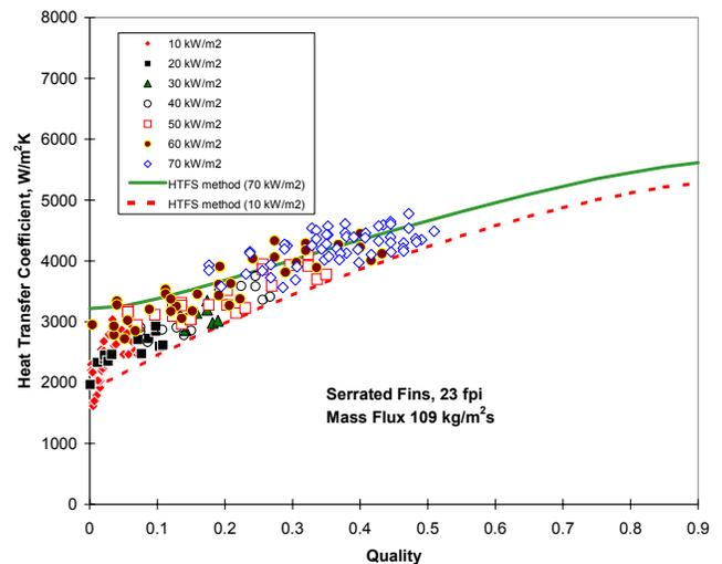
Fig. 4 Predictions of the HTFS method and recent HTFS data for flow boiling of pentane (Wadekar, 2002)
