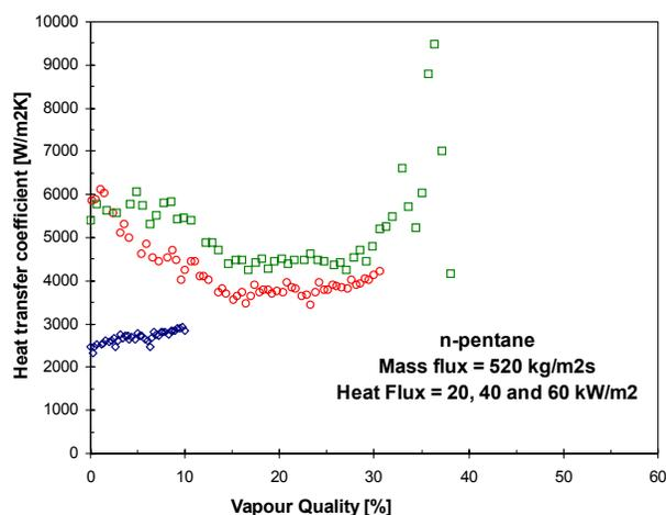
Fig. 2 Flow boiling heat transfer in a 25.4 mm i.d. tube at different heat fluxes
