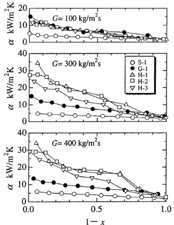
Fig. 6 Performance of plain, helical and herringbone microfin tubes for condensation (Miyara and Otsubo, 2001)
