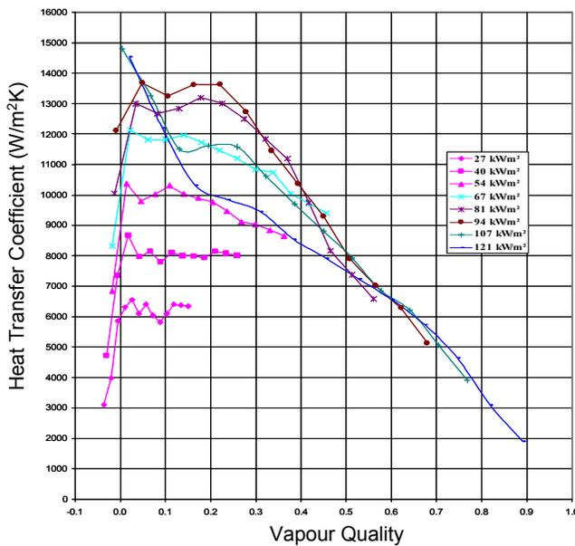
Fig. 3 Flow boiling heat transfer in a 2.01 mm i.d. tube at different heat fluxes (mass flux = 300 kg/m<sup>2</sup>s, pressure = 8 bar) from Huo et al (2003)
