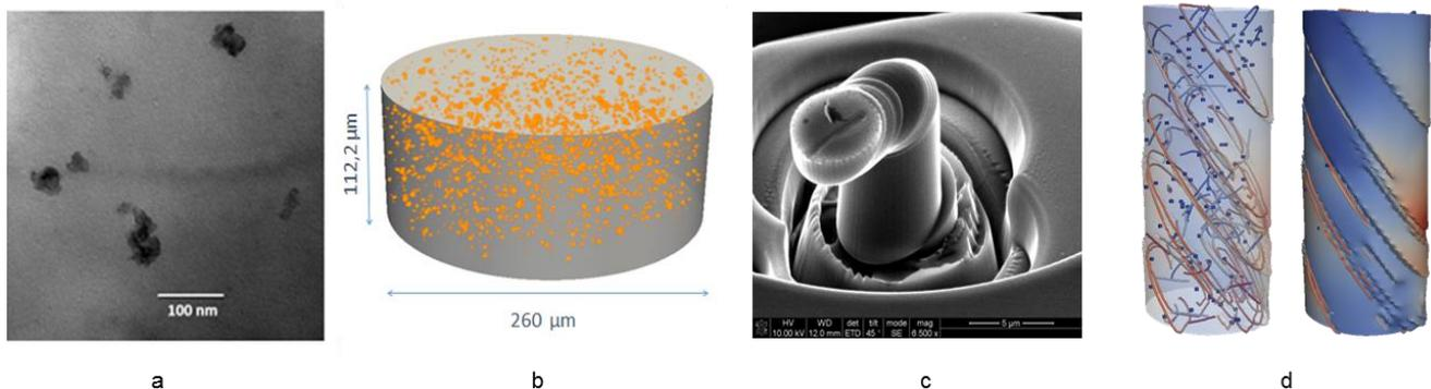
Figure 1 - TEM micrograph showing the  $\text{Y}_2\text{O}_3$  particles in the FSPed sample (a). Synchrotron X-ray microtomography confirms the homogeneous dispersion of particles (b). Post-compression structure (c). 3D dislocation dynamics simulations of a micropillar ( $\varnothing=10 \mu\text{m}$  and  $h=25\mu\text{m}$ ) with cubic particles ( $f_v=0.1\%$  and  $\varnothing=250\text{nm}$ ) (d).
