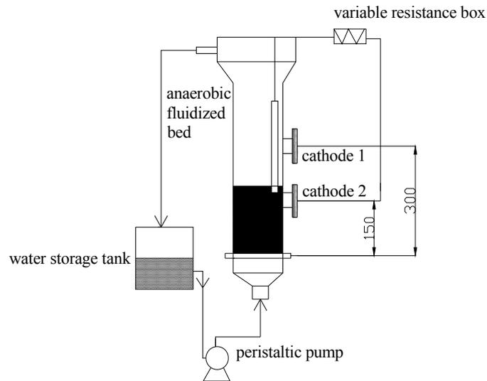
Figure 1 The schematic of Anaerobic fluidized bed MFC
