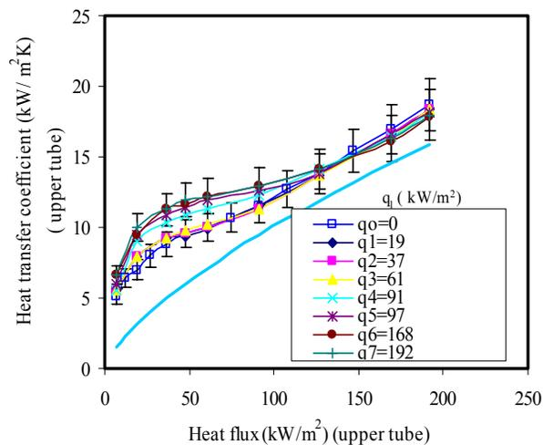
Fig 3: Variation of heat transfer coefficient with heat flux with distilled water as working fluid.
