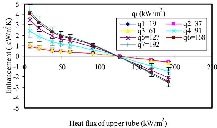
Fig. 8: Correlated plot of enhancement against heat flux for upper tube
