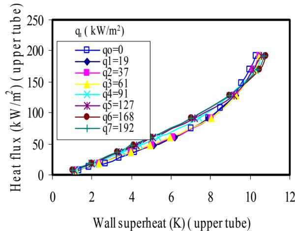
Fig 2: Variation heat flux with wall superheat with distilled water as the working fluid
