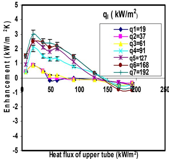
Fig 5: Variation of enhancement against heat flux of upper tube for distilled water
