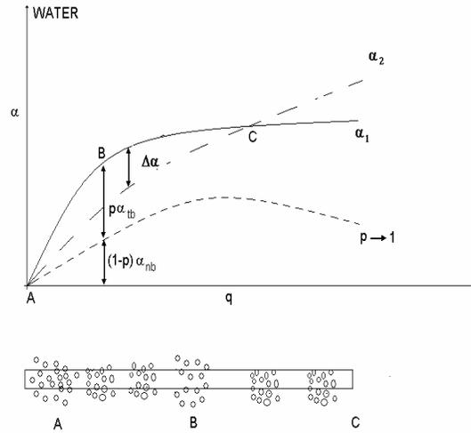
Fig. 4: Diagram showing the superimposition model for boiling of the upper tube
