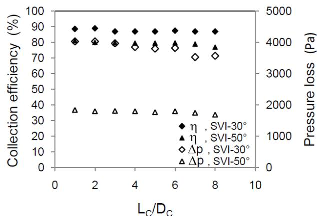
**Fig. 4.** Performance data of Uniflow Cyclone type 1 as a function of separator length  $L_C$  (Carolith 20-R,  $L_{VF}=0$ mm).
