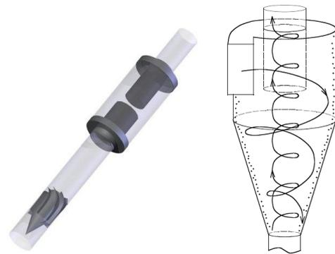
**Fig. 1.** Uniflow cyclone (left) and standard reverse flow cyclone (right).
