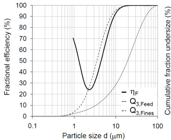
**Fig. 9.** Fractional separation efficiency of Uniflow Cyclone type 2B ( $L_C/D_C = 3.6$ , Carolith 20-R,  $\eta = 88.6\%$ ,  $\Delta p = 2510 \text{ Pa}$ ). Dashed curves: Cumulative fractions undersize of feed and fines (Measurements by Laser Diffraction).
