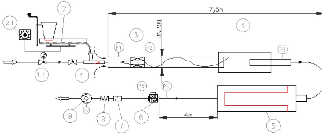
**Fig. 2.** Scheme of the test plant. 1. Injector (1.1 pressurized air), 2. Vibrating feeder (2.1 Potentiometer for mass flow control), 3. Swirl generator, 4. Dust bunker, 5. Filter, 6. Orifice measuring the gas flow rate, 7. Sound absorber, 8. Compensator, 9. Radial fan.
