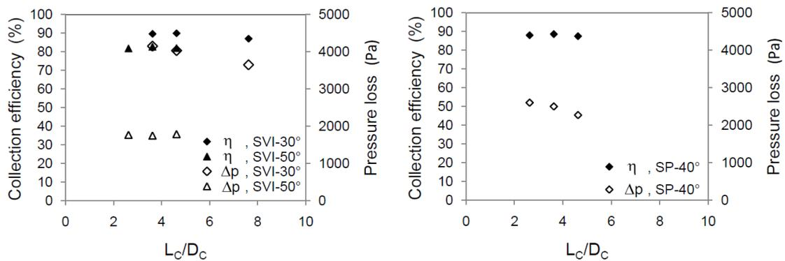
**Fig. 7.** Performance data of Uniflow Cyclone type 2A (left) and type 2B (right) as a function of separator length  $L_C$  for swirl generators SVI-30° and SVI-50° (both types with Carolith 20-R,  $L_{VF} = 400$  mm, without core).
