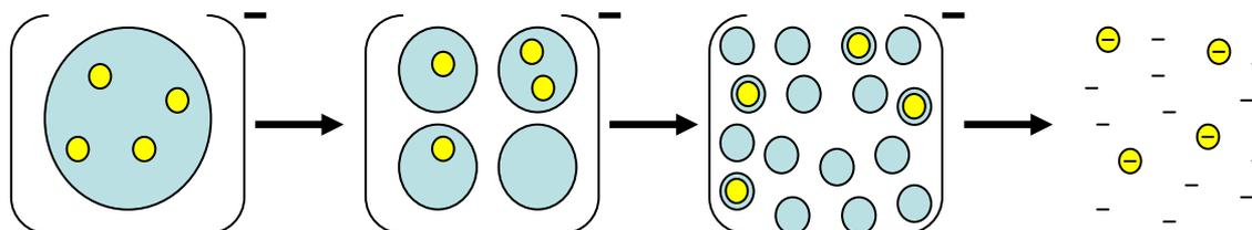
Figure 1. Scheme of scattering mechanism in nanosuspension EHDA. Left: a charged liquid droplet seeded with nanoparticles. Middle: the droplet shrinks due to liquid evaporation and Rayleigh break up. The nanoparticles are distributed over the new generated droplets after each Rayleigh break up. Right: upon total drying a spray of charged nanoparticles is obtained.
