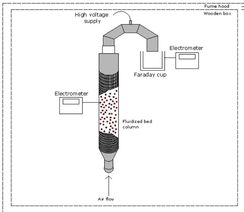
Figure 4 Experimental set-up for elutriation and capture of charged host particles.
