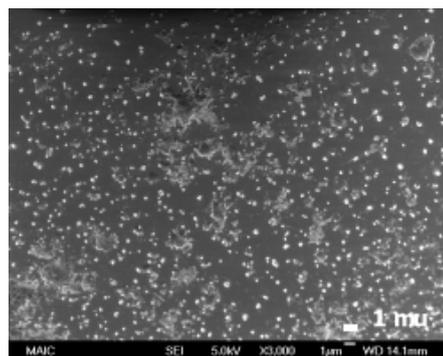
Figure 6. SEM image of 500 nm polystyrene particles deposited with electro spraying on a falling flow of 200  $\mu\text{m}$  glass beads.
