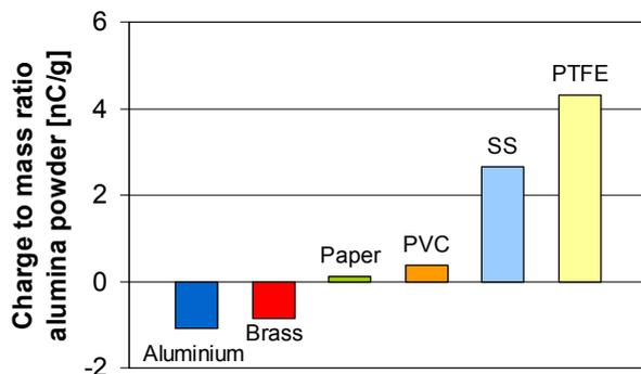
Figure 2. Determined tribo-series of alumina powder by simple experiments. Charge to mass ratio based on accumulated charge of alumina samples with given mass. (PVC = polyvinylchloride, SS = stainless steel, PTFE = polytetrafluorethylene.)
