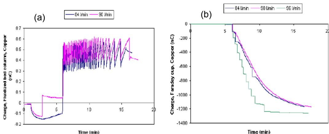
Figure 5. (a) Effect of gas velocity on the net charge in the fluidized bed column; (b) charge accumulation in the external Faraday cup from collecting the entrained particles (5 min fluidization and 10 min elutriation).
