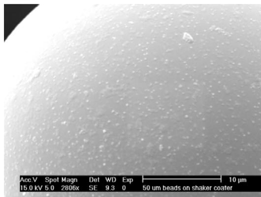
Figure 3. SEM image of 50 micron glass beads coated with 100 nm nanoparticles.
