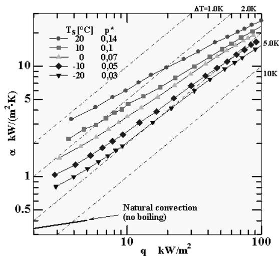
Figure 5: Boiling heat transfer coefficient on one coated tube (Effect of pressure)
