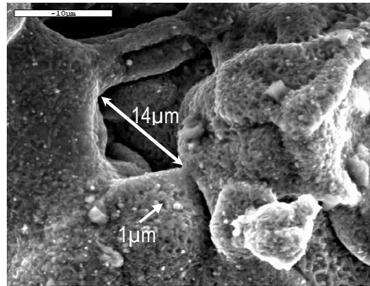
Figure 2: SEM picture of the Copper coating 3500:1
