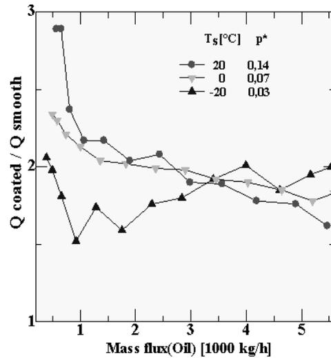
Figure 10: Enhancement of the transferred heat per coated tube
