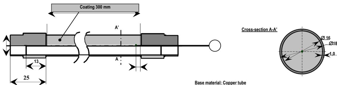
Figure 1: Detail of the test tube
