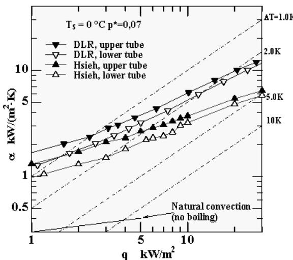
Figure 8: Boiling heat transfer of two 2\*2 tube bundle with different coating parameter
