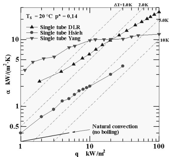
Figure 6: Boiling heat transfer on several porous coated tubes in the literature
