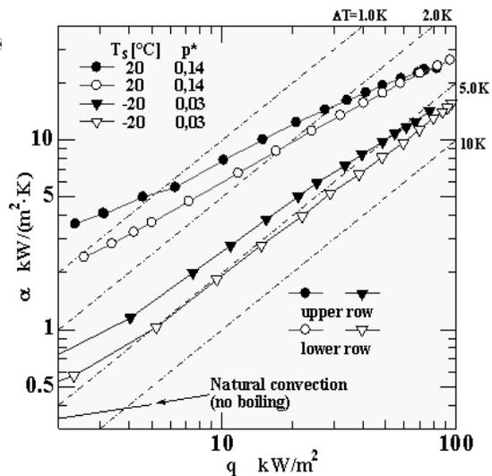
Figure 9: Boiling heat transfer on the upper and lower row of a 2\*2 tube bundle
