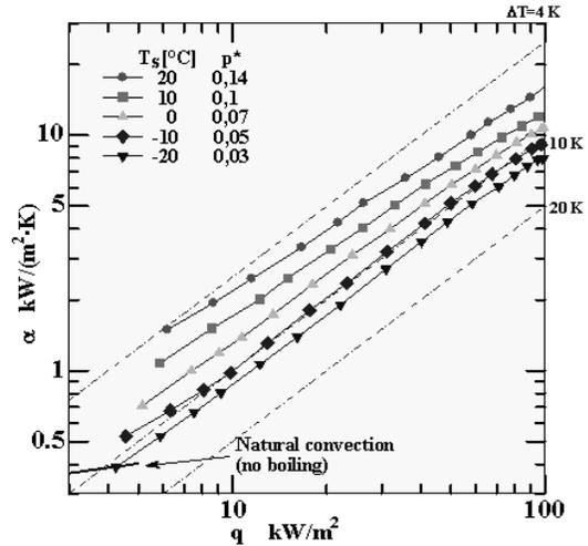
Figure 4: Boiling heat transfer coefficient on one smooth tube (Effect of pressure)
