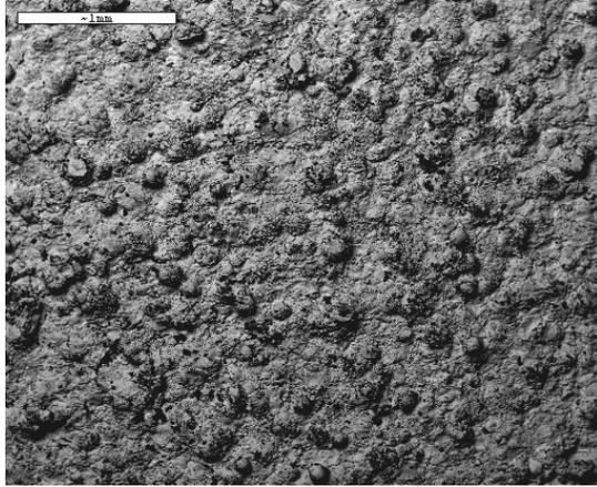
Figure 3: SEM picture of the Copper coating 35:1
