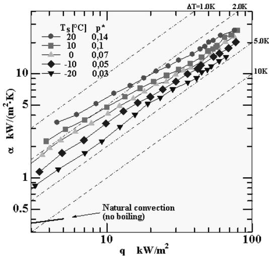
Figure 7: Heat transfer on the upper of two tubes
