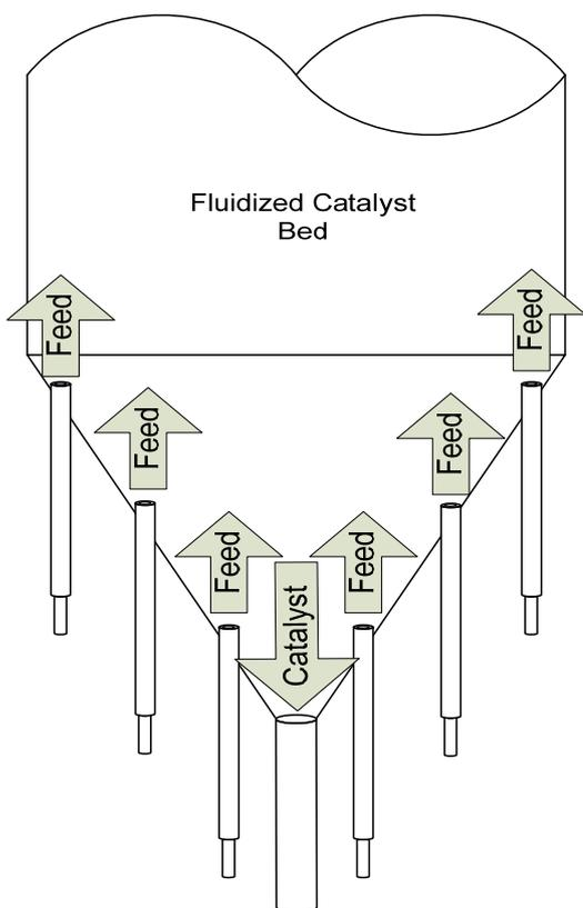
**Figure 1: Cone Design Grid**
