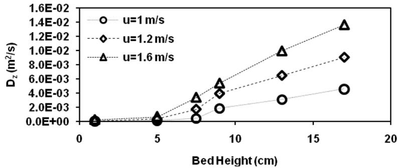
**Figure 3:** Axial diffusivity of particles at different gas velocities for a bed of mono-charged particles as a function of height,  $q = 50$  pC
