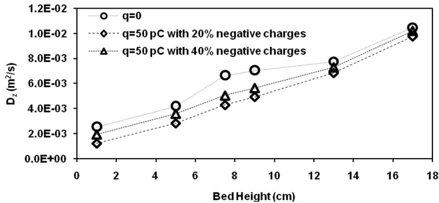
**Figure 4:** Axial diffusivity of particles at different gas velocities for a bed of bi-polar charged particles as a function of height,  $q = 50$  pC
