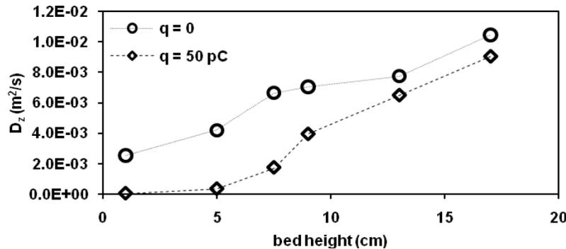
Figure 2: Axial diffusivity of particles for neutral and mono-charged bed as a function of height,  $U_0 = 1.2 \text{ m/s}$
