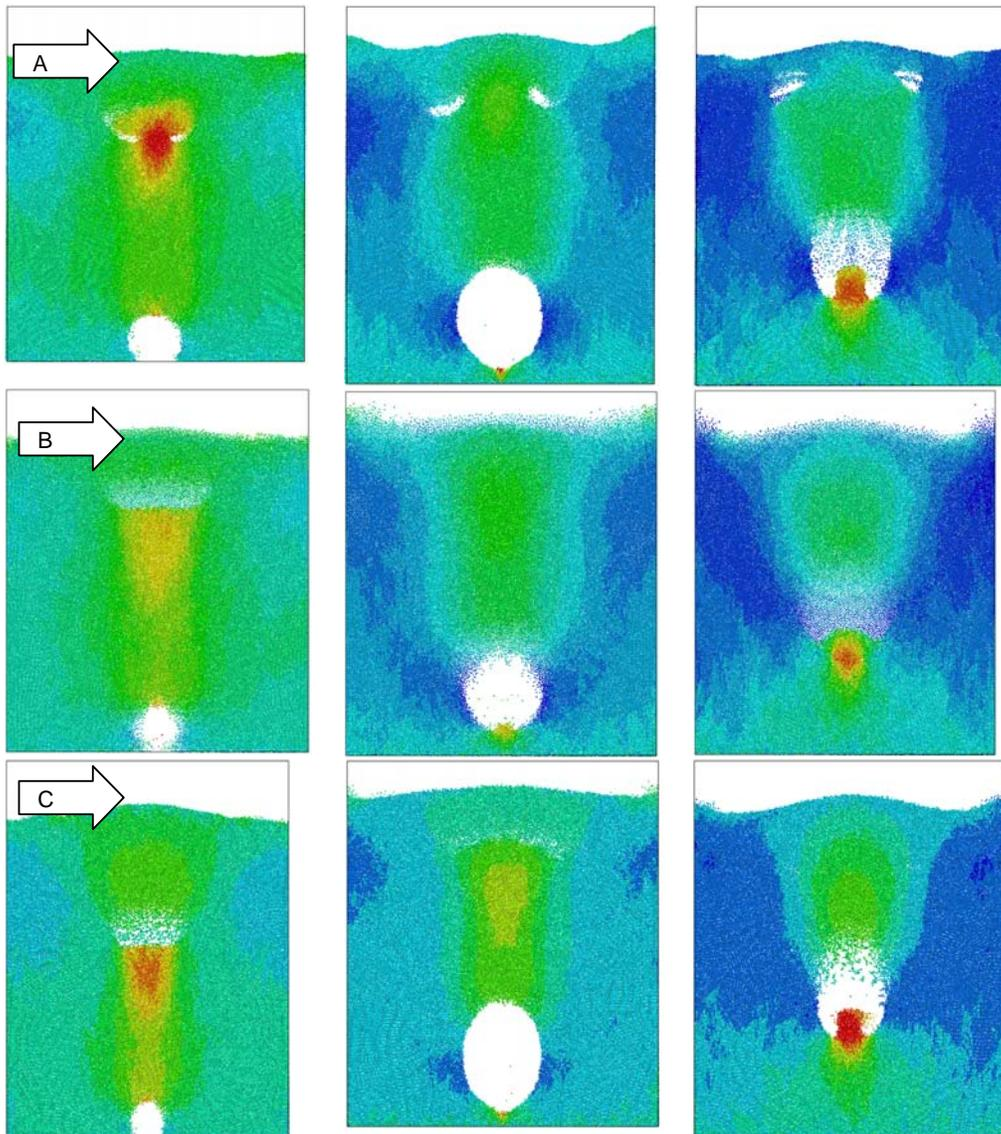
**Figure 1** Bubble formation and motion in a bed with (A) neutral, (B) mono-charged ( $q=50$  pC) and (C) bipolar charged ( $q=50$  pC with 40% negative and 60% positive charged particles) particles
