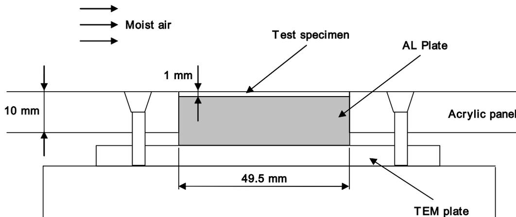
Fig. 2 Schematic diagram of TEM and test plate.
