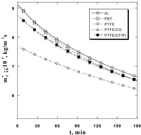
Fig. 6 Temporal variations of mass transfer for different test specimens.
