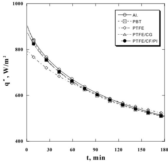
Fig. 5 Temporal variations of heat transfer for different test specimens.
