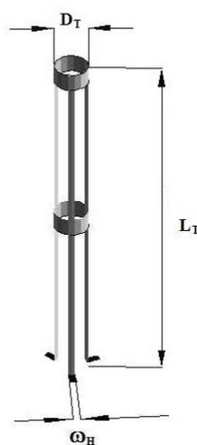
**Figure 3.** Scheme of the open-sided draft tube.
