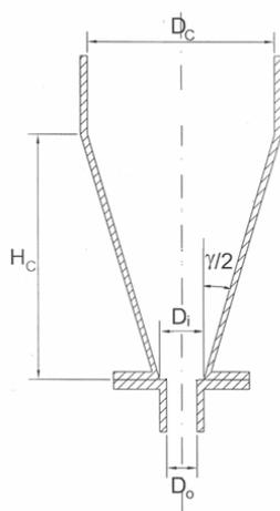
**Figure 2.** Geometric factors of the conical contactors.
