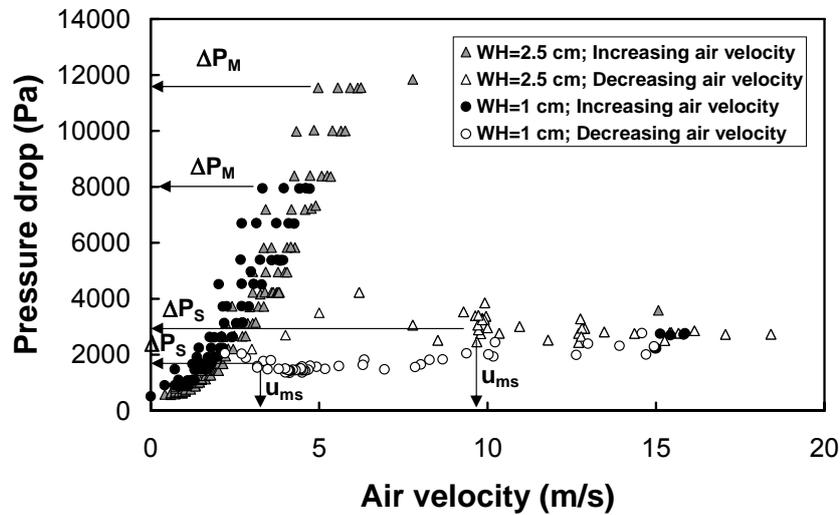
**Figure 5.** Evolution of the bed pressure drop with air velocity for different values of the widths of the faces ( $\omega_H$ ) when non-porous draft tubes are used. Experimental conditions:  $\gamma=36^\circ$ ;  $D_0=0.04$  m;  $H_0=0.25$  m,  $D_T=0.042$  m.
