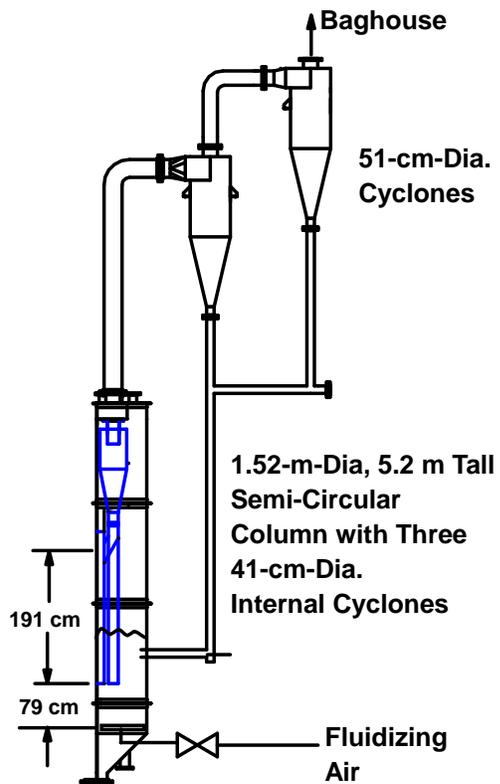
Figure 1. Side View of the Test Unit
