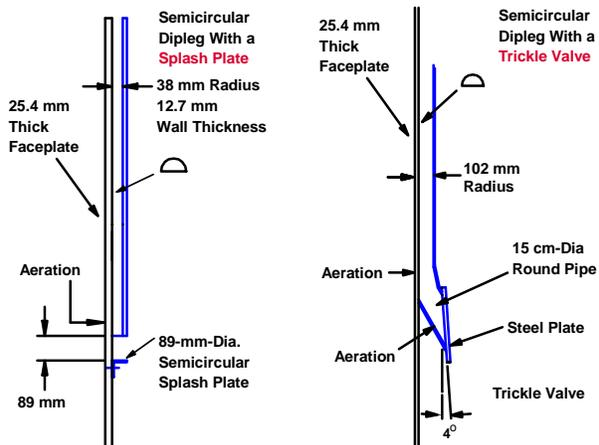
Figure 3. Schematic Drawing of Diplegs with a Splash Plate and a Trickle Valve
