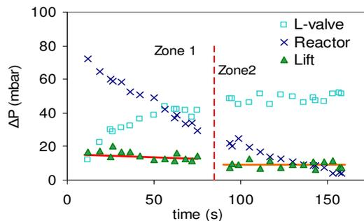
**Figure 5:** Pressure drop evolution in the standpipe of the I-valve for a batch solid circulation from R1 to R2 with  $Q_{IV} = 0.18 \text{ Nm}^3/\text{h}$ ,  $G_s = 196 \text{ kg/m}^2.\text{s}$  in zone 1 and  $98 \text{ kg/m}^2.\text{s}$  in zone 2 (right).
