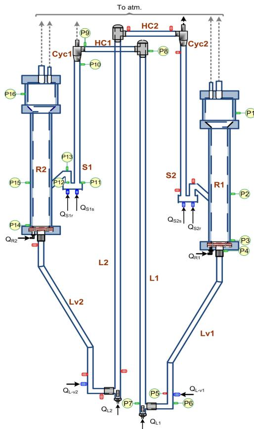
**Figure 1: Scheme of the CLC cold flow prototype ,Gas injection and pressure measurement taps are indicated .**
