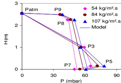
Figure 7: Model prediction of pressure evolution for different heights in the prototype.
