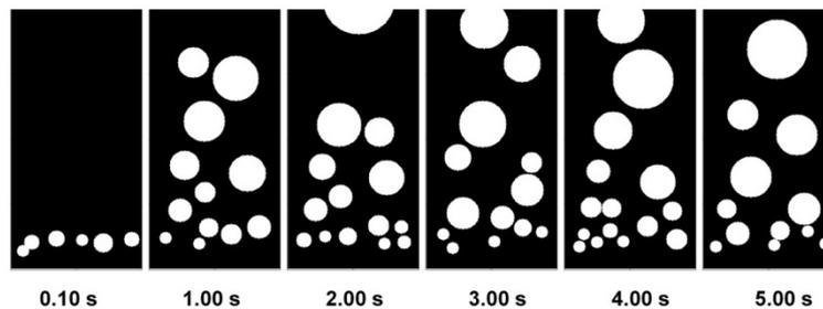
**Figure 1:** Graphical representation of simulated bubbles at  $U = 18$  cm/s.
