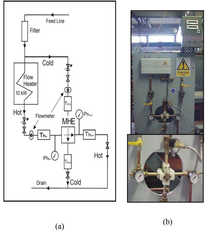
Figures 8 (a) and (b): Flow loop test rig schematic.
