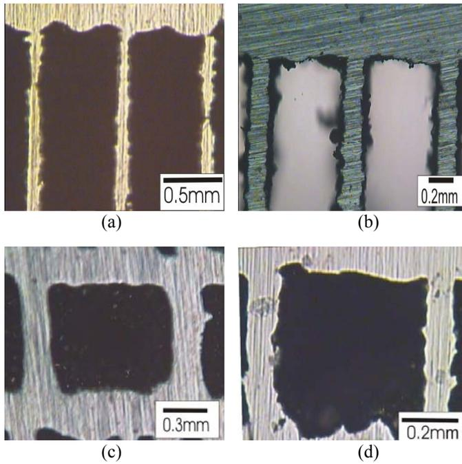
Figure 9 (a), (b), (c) and (d): Micrographs of micro channel heat exchangers by SLM.
