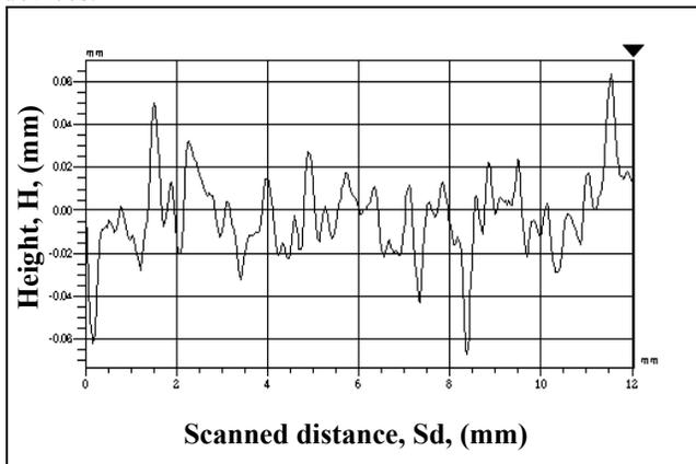
Figure 10: Roughness plot for Ra of 12  $\mu\text{m}$ .
