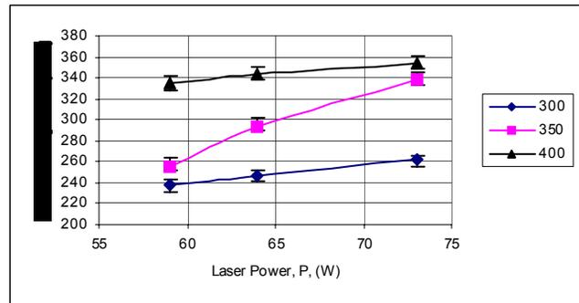
Figure 6: Tensile strength characteristics for Selective Laser Melted 316L stainless steel.
