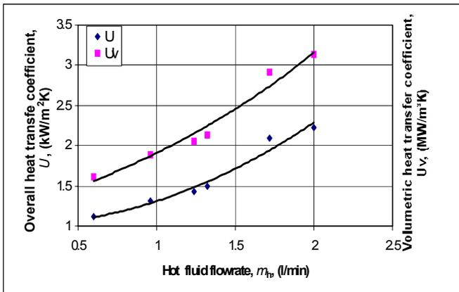
Figure 12: Overall and volumetric heat transfer coefficient as function of the hot side.
