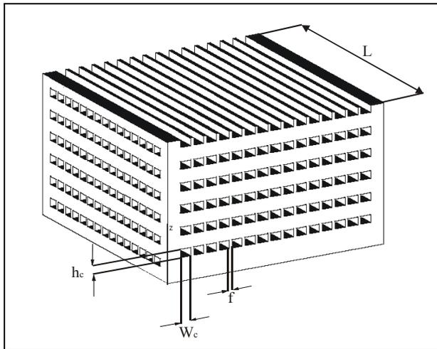
Figure 2: Basic Schematic of a Cross Flow Heat Exchanger.
