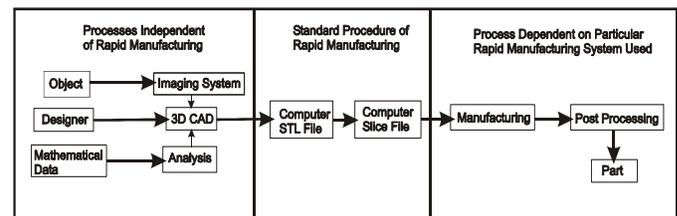
Figure 4: Basis of Rapid Manufacturing Processes, (Murphy et al. 1995).
