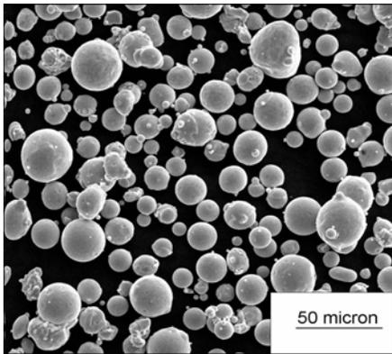
Figure 7: SEM picture of powder.
