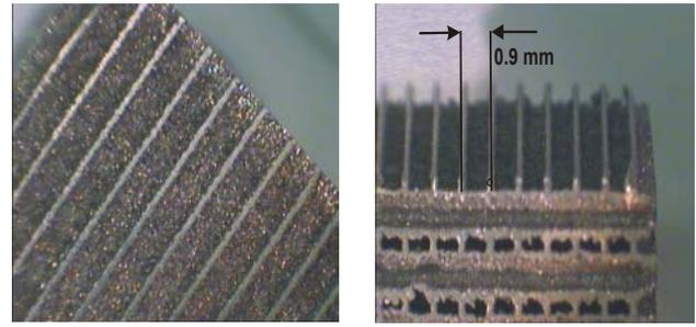
Figure 11: Frame of a typical micro cross-flow heat exchanger by SLM.
