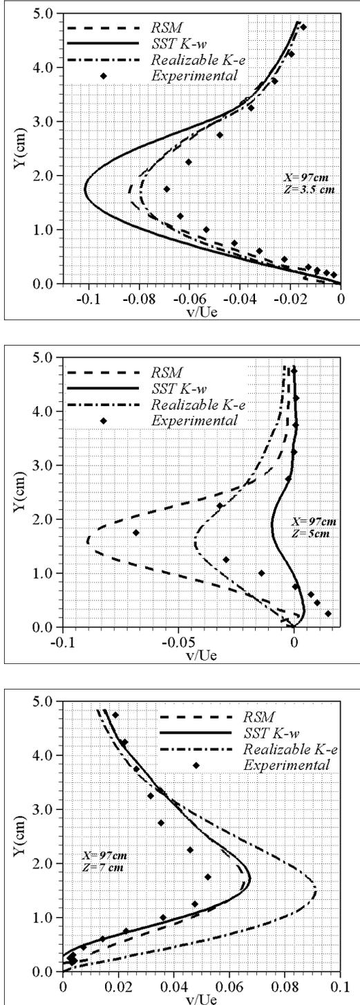
Figure 6. Normalised vertical velocity profiles ( $v/U_e$ ) at  $X = 97\text{cm}$  at different  $Z$  locations
