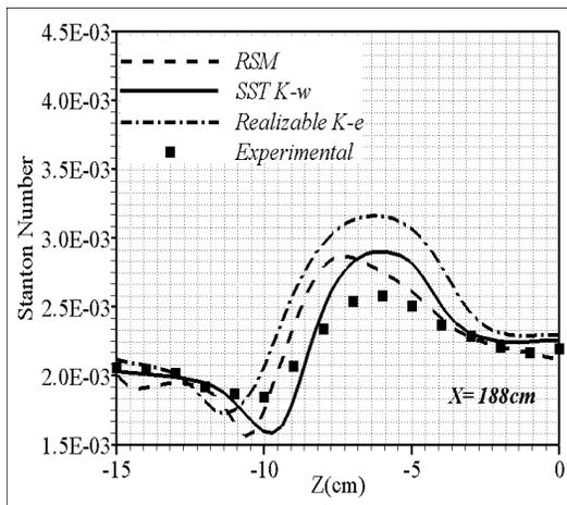
Figure 7. Spanwise distribution of Stanton Number at different X locations
