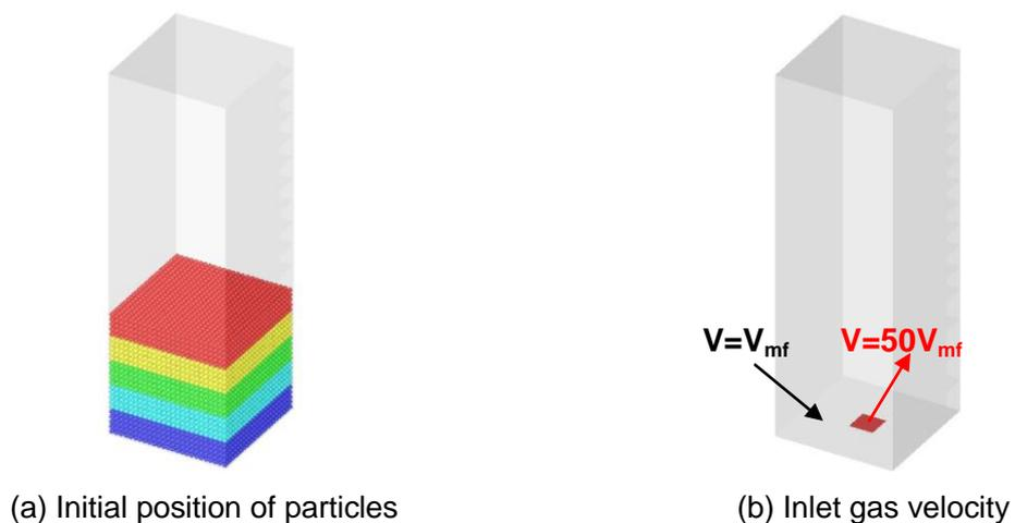
Fig.3 Boundary condition and Initial condition
