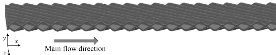
Fig. 1: Geometrical domain for PHE with  $\beta = 60^\circ$ .
