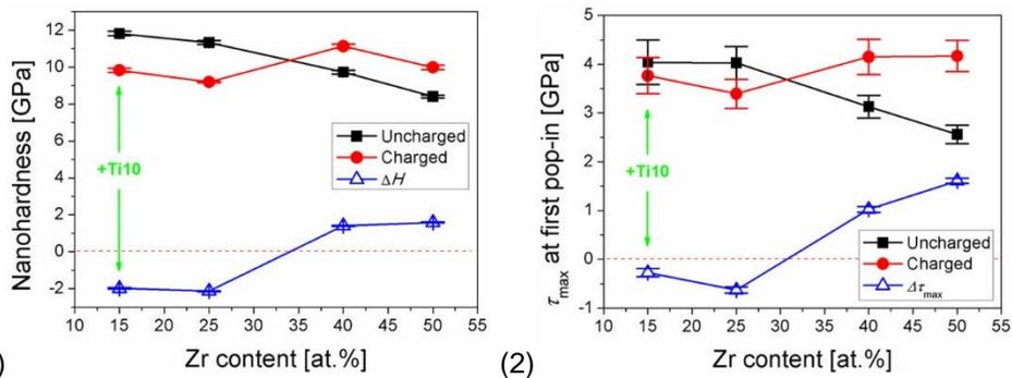
Figure 1. Variations in (1) hardness ( $H$ ) obtained from cube-corner nanoindentation and the hydrogen-induced change ( $\Delta H$ ), and (2) the maximum shear stress ( $\tau_{max}$ ) at the first pop-in obtained from spherical nanoindentation and the hydrogen-induced difference ( $\Delta \tau_{max}$ ) with Zr content. The data of Zr15Ti10 are identified as “+Ti10”.
