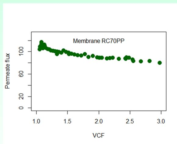
Fig. 2 Variation of permeate flux (L h<sup>-1</sup> m<sup>-2</sup>) with VCF for membranes RC70PP
