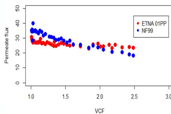
Fig. 3 Variation of permeate flux (L h<sup>-1</sup> m<sup>-2</sup>) with VCF for membranes ETNA01PP and NF99
