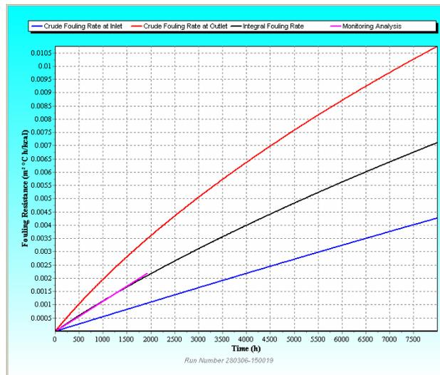
Fig. 2 Predicted Fouling Rates for Exchanger T29
